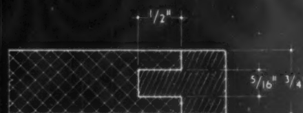
grooved to receive hardwood lipping
