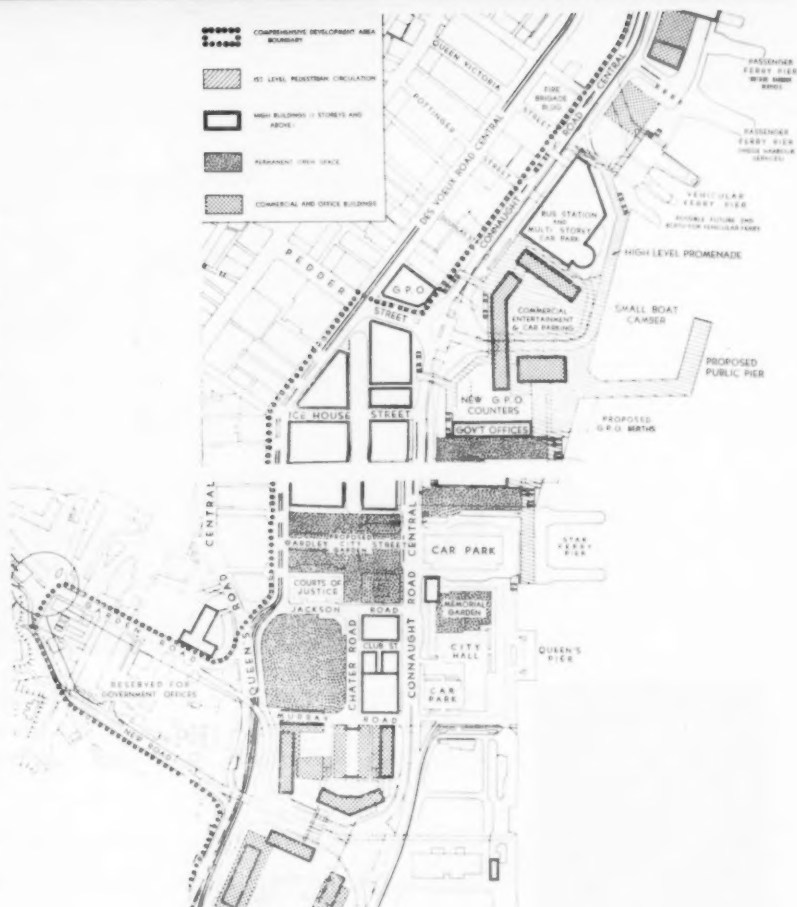
Hongkong's projected city centre development: above, the model from the harbour; right, a keyed plan of the project, showing tall buildings, pedestrian circulation areas, open space and area zoned for commercial and office buildings
