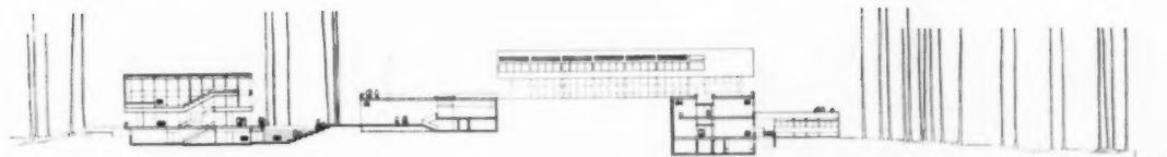
Section through auditorium block, open air theatre, gymnasium block and science block
