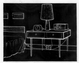
The 13 amp socket outlet and fused plug has been designed particularly for use on ring circuits and is ideal where single outlets only are required.
