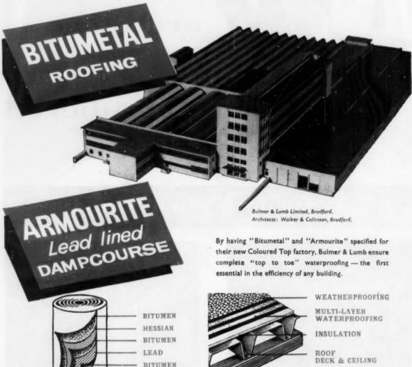
"Armourite" Dampcourse, reinforced with a lining of sheet lead, gives that "extra" protection required in good class building construction. Available in 4 grades. Standard—8 lbs; 7B—10 lbs; 10C—12½ lbs; Super Heavy—18 lbs. per sq. yd. Lead Content 4 ozs, 7 ozs, 10 ozs. and 16 ozs. per sq. ft.
