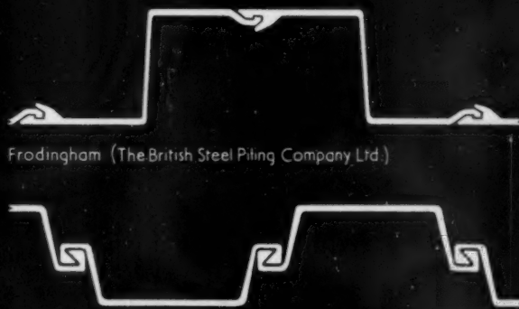
Larssen (South Durham Steel and Iron Company Ltd.) STEEL SHEET PILES: TYPICAL PROFILES
