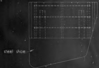
elevation of toe CONCRETE SHEET PILES
