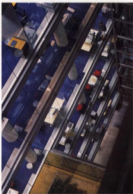
Above: chilled beams give a strong character to workspaces, dispelling the depressing blandness induced by suspended ceilings. Below: naturally ventilated lightweight glazed atria act as climatic buffers, mediating between the external climate and that of the offices
