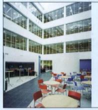
Halifax' latest call centre in Belfast is being protected by FendorHansen, which supplied and installed its Fineline fire-resistant glazing system to create the large central glass atrium. Combined with 6mm Pyrolithic glass, Fineline screens offer minimum slightlines and 30minutes integrity fire performance.
