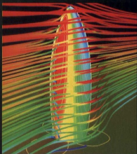
Above: airflows around the building assist the internal ventilation and are predicted to benefit the local micro-climate
