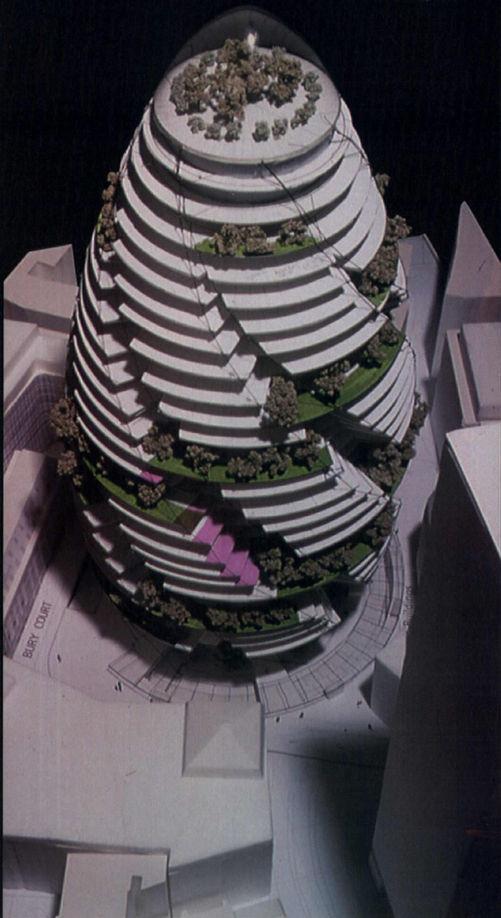
Key model of the storey arrangement, showing bioclimatic terraces and cutaway voids
