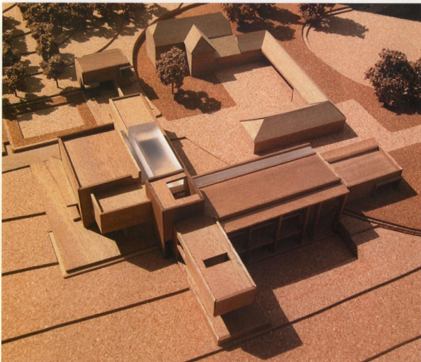
Top: proposed site plan. Above: the model, showing the projecting master bedroom, winter garden (shown as clear block) and top-lit corridor
