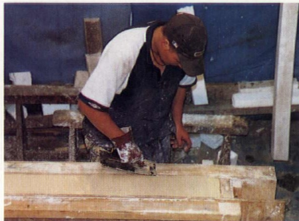
Trowelling is the final smoothing process. Note that protective facial equipment is not deemed necessary
