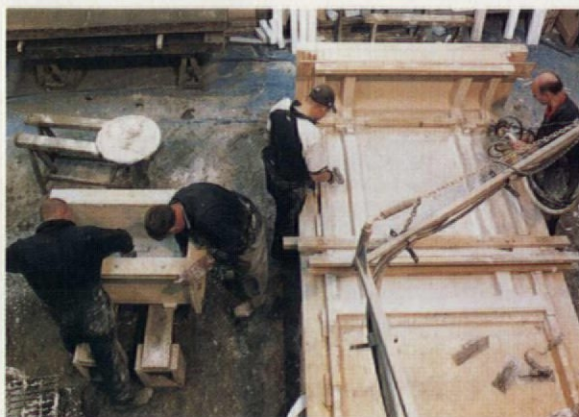
During curing of a cladding panel, the GRC is rolled by hand
