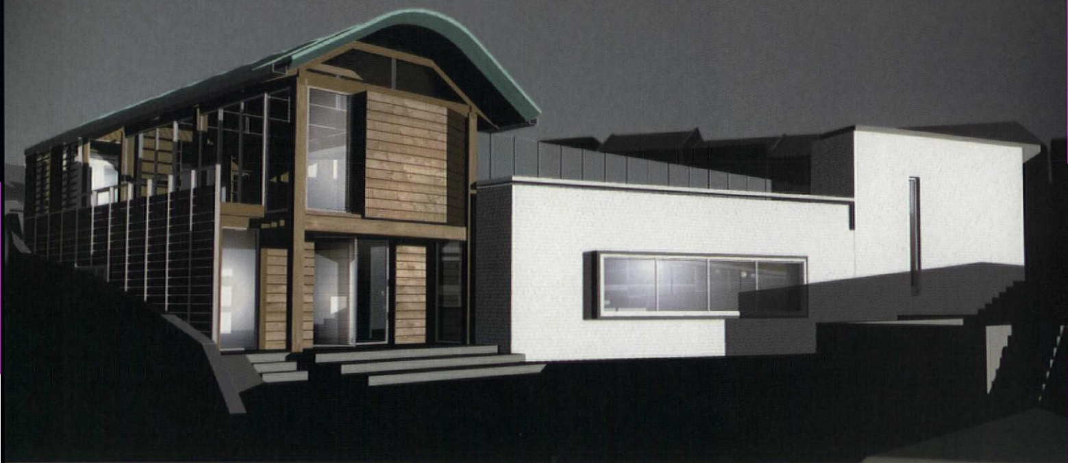
The architect's earlier CAD image from the north (pool then not adjacent to house). The north-east, larch-clad facade is tight to the site boundary
