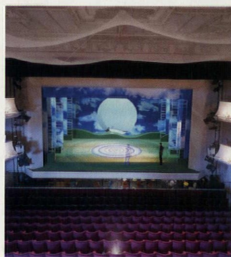
There are two levels of boxes. The new soffitt is fibre optic-lit, while the existing ceiling is netted. The upper boxes have flush jib doors
