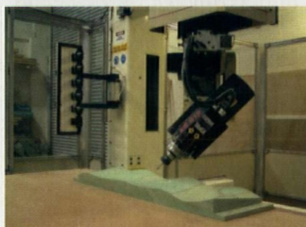
Above: many elements are curved and contain inlays and contouring with individual patterns. Right: three-dimensional computer models were translated into moulds for the poured concrete
