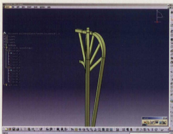
Left: isometric view of one of the 24 primary columns that support the roof and facade
