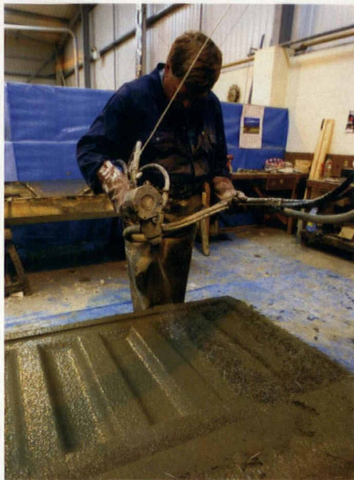
Compressed air forces the GRC mix on to the mould
