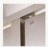
Door formed from 0.7mm anodised aluminium, factory folded on leading edges and bonded to a 25mm core.
