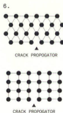
6. Ideogram of nuclei/ bond array in ductile and brittle materials. Ductile: cracking is prevented by the nuclei backing the bond. Brittle: nothing stops the crack developing – the more bonds break, the more stress is concentrated on the crack
