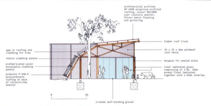
10. Cross section through the viewing enclosure
