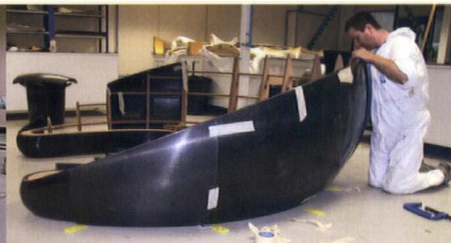
7. Skeleton made from 18mm marine-grade ply components, cut with a CNC router. Finished panels bonded to frame with epoxy to produce rigid shell structure
