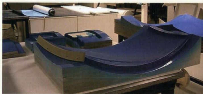
5. Two pre-impregnated carbon-fibre sheets plus a flexible foam core are formed around the moulds, using a process of vacuum forming and oven baking in an autoclave to create a 25mm-thick stressed-skin laminated composite panel of carbon, foam and carbon
