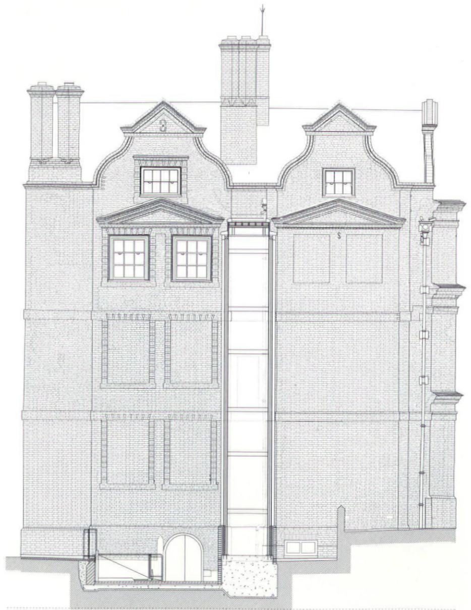
6. Section through new lift shaft and platform lift to basement showing west elevation
