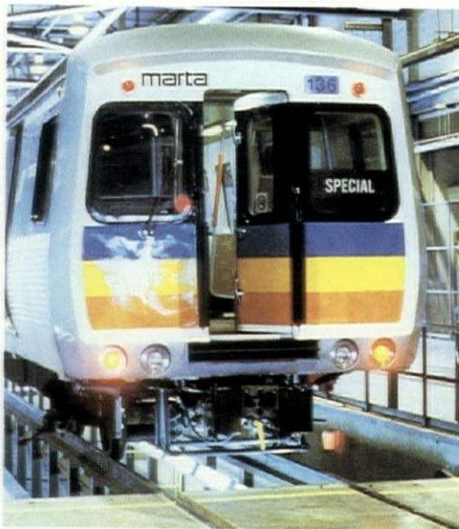
During any eight-hour shift, as many as 50 railcars can rumble into the MARTA car shop for routine repairs, regularly scheduled preventive maintenance, or inspection. The Metropolitan Atlanta Transit Authority inspects each of its railcars every 45 days with progressively increasing detail. A 45-day inspection takes about four hours, says Dan Estep, chief of vehicle maintenance at MARTA. Ninety-day and semiannual inspections take longer. Annual inspections take from 8 to 10 hours, Estep says.
