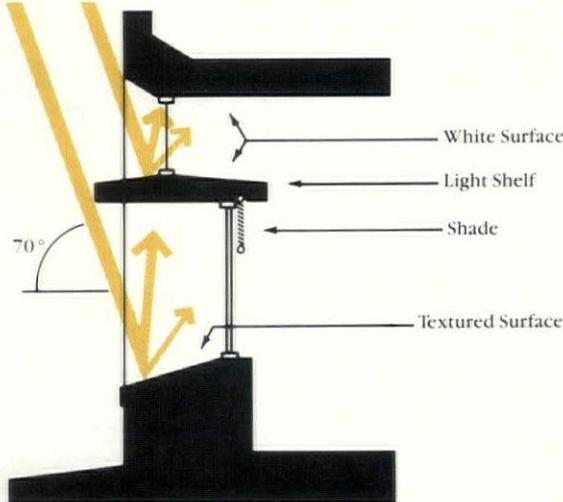
Light shelves can bounce sunlight deep into a building. Under cloudy sky conditions, daylight may not meet task lighting needs, yet provide adequate ambient light.
