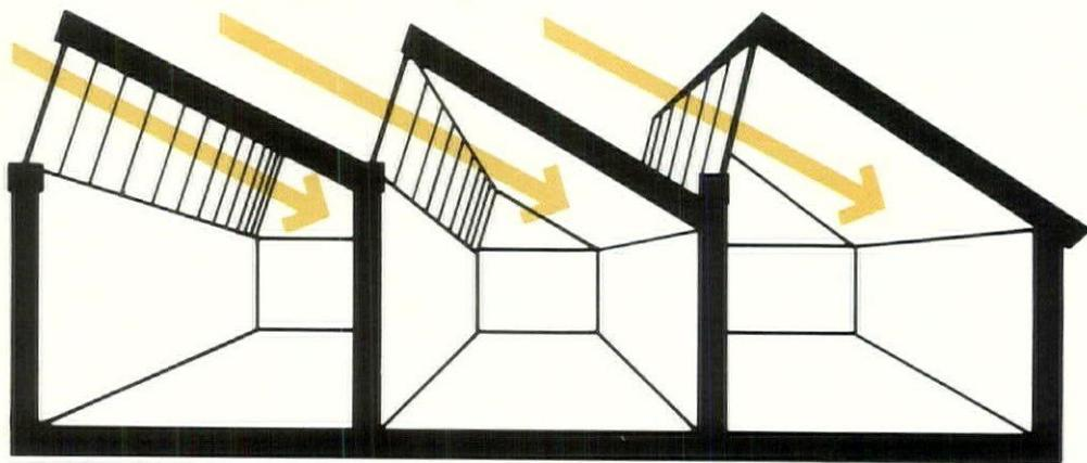
*Roof monitors were once used much more frequently than they now are. The better examples of roof monitors excluded most direct radiation, a function of glazing orientation and geometry.*
