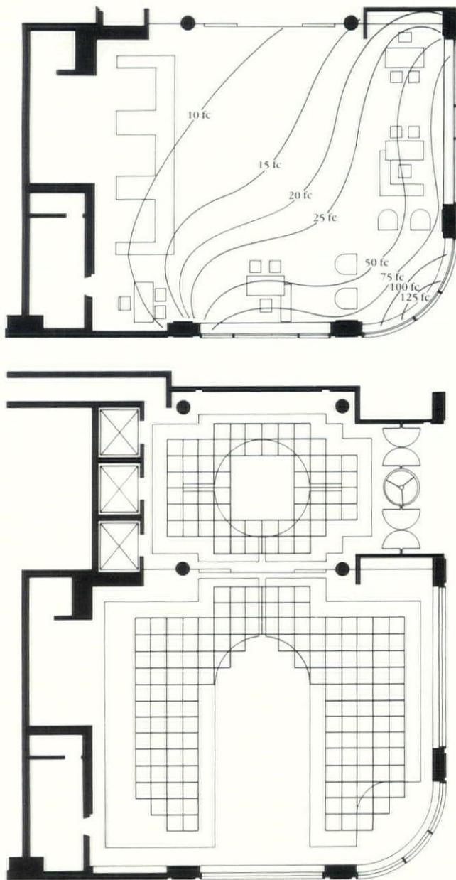
*Isofootcandle contours show the illumination contribution of daylight from a typical overcast Seattle sky through the full-height window wall. The reflected ceiling plan shows the layout of the neon grid.*
