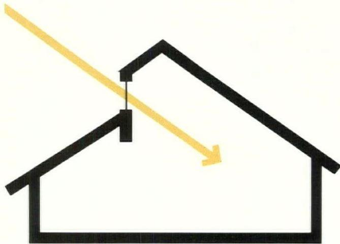
*Southern-oriented roof monitors diffuse and direct light into the interior spaces and provide winter heat. High ceilings allow openings for natural ventilation.*
