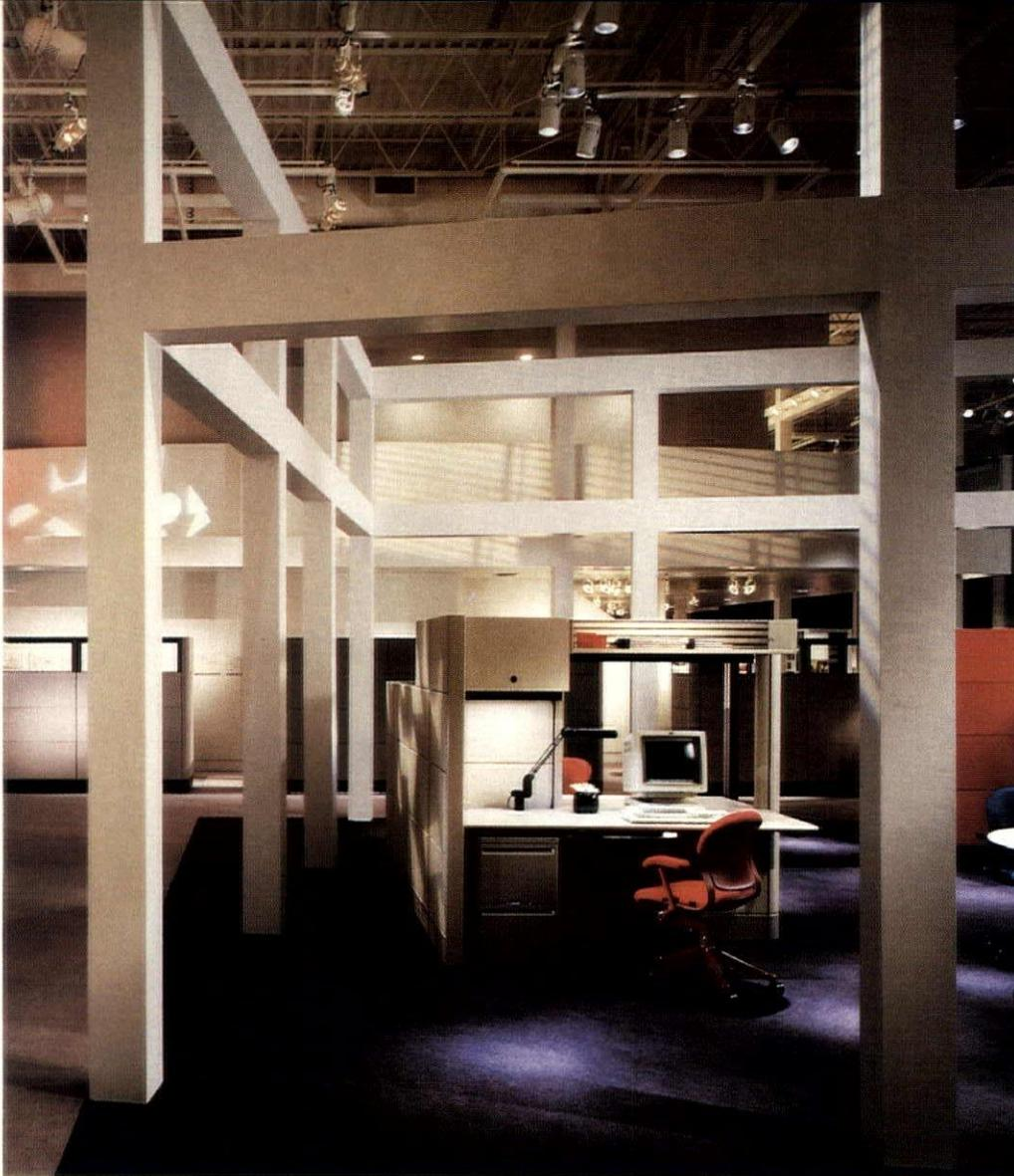
*The 3:1 average brightness-contrast ratio between display and ambient lighting gives extra "punch" to product displays.*
