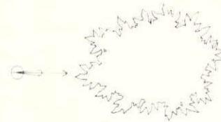
Large, open-form trees require 5, 10, or more fixtures to cover the entire canopy area, as shown with this California live oak (*Quercus agrifolia*). The aiming angle is from 10 degrees to 35 degrees; one fixture, shown at far left, is aimed straight up at the edge of the canopy.
