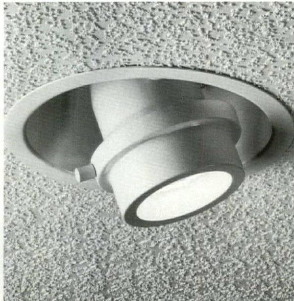
**THE 281 SERIES SEMI-RECESSED SPOTLIGHT FROM LIGHTING SERVICES** is designed to accommodate 50- and 70-watt PAR 30 tungsten-halogen medium screwbase lamps and is available with glass color filters, spread lenses, and light blocking screens. The series is featured in LSI black, white, and silver aluminum finishes. Lighting Services, Inc., Stony Point, NY. *Circle No. 60 on product card.*
