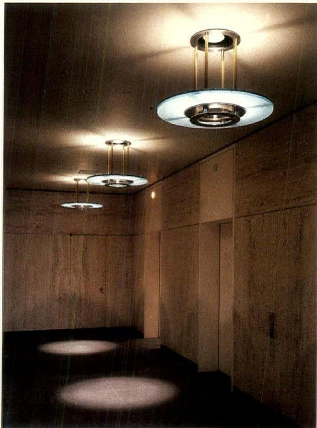
**INTERSECTING CIRCLES:** Pendants are positioned so direct downlight from 250-watt quartz PAR 38s strikes the intersection of four 2.5-foot slabs of granite flooring.
