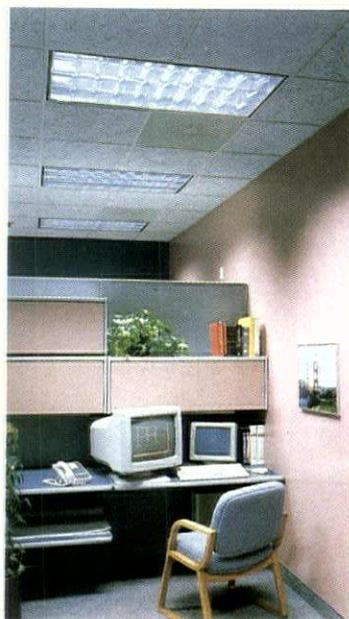
▶ **THE OPTIMAX LIGHT CONTROL SYSTEM FROM LITHONIA LIGHTING** is a fluorescent lighting system that eliminates glare, and provides appropriate levels of general illumination for tasks. This recessed parabolic, with a specular aluminum louver designed to direct light away from glare-producing angles, provides a uniform level of 70 maintained footcandles of illumination. This system is available in 2-foot x 4-foot and 2-foot x 2-foot models. Lithonia Lighting, Conyers, GA. **CIRCLE 48**
