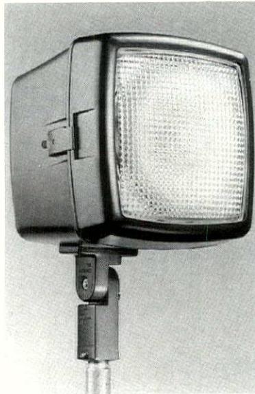
**GTE'S SYLVANIA WATCH-KAT** unit generates infrared light rays that can be seen by standard closed circuit TV cameras. The device is approximately 9 inches cubed and comes with three lens configurations of narrow spot, medium flood, and wide flood. The fixture lamp is rated at 300 watts and has an average life of 4,000 hours. GTE Security Lighting, Fall River, MA. **CIRCLE 40**
