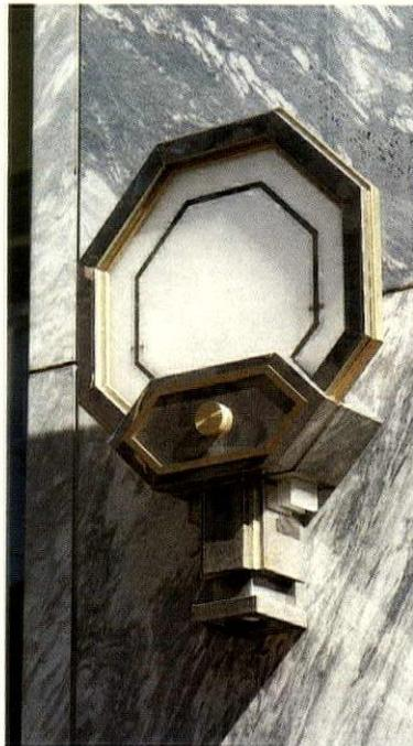
CHICAGO'S WATERTOWER PLACE EXTERIOR OCTAGON WALL SCNCE is manufactured by Appleton Lamplighter and designed by Green Hiltcher, Shapiro. The fixture measures 32 inches x 44 inches with a 9-inch projection. The fixture is made of polished stainless and satin bronze, and the frosted lens is backlit with white neon. A 250-watt quartz lamp provides downlight. Appleton Lamplighter, Appleton, WI. **CIRCLE 46.**
