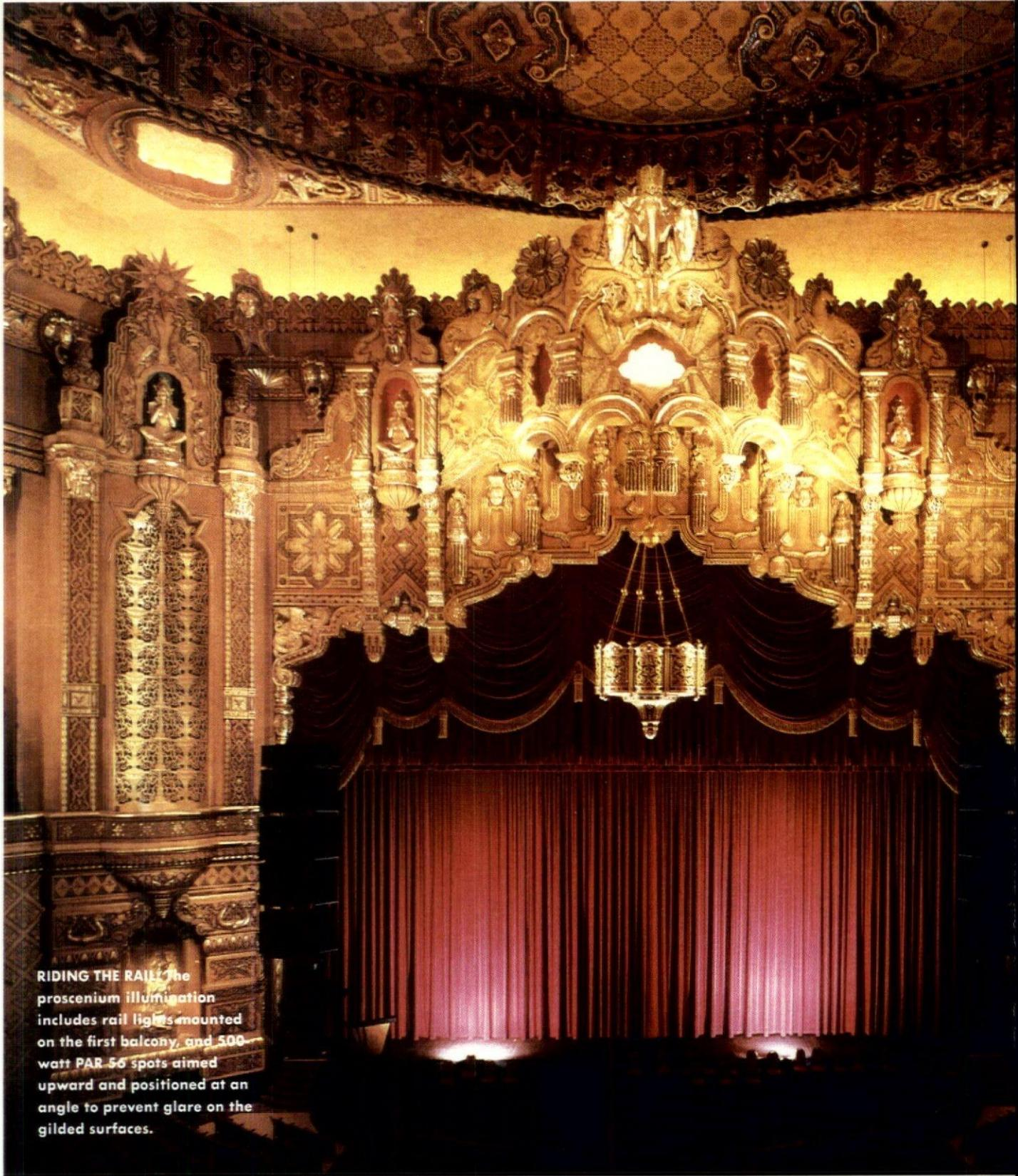
**RIDING THE RAIL:** The proscenium illumination includes rail lights mounted on the first balcony, and 500-watt PAR 56 spots aimed upward and positioned at an angle to prevent glare on the gilded surfaces.
