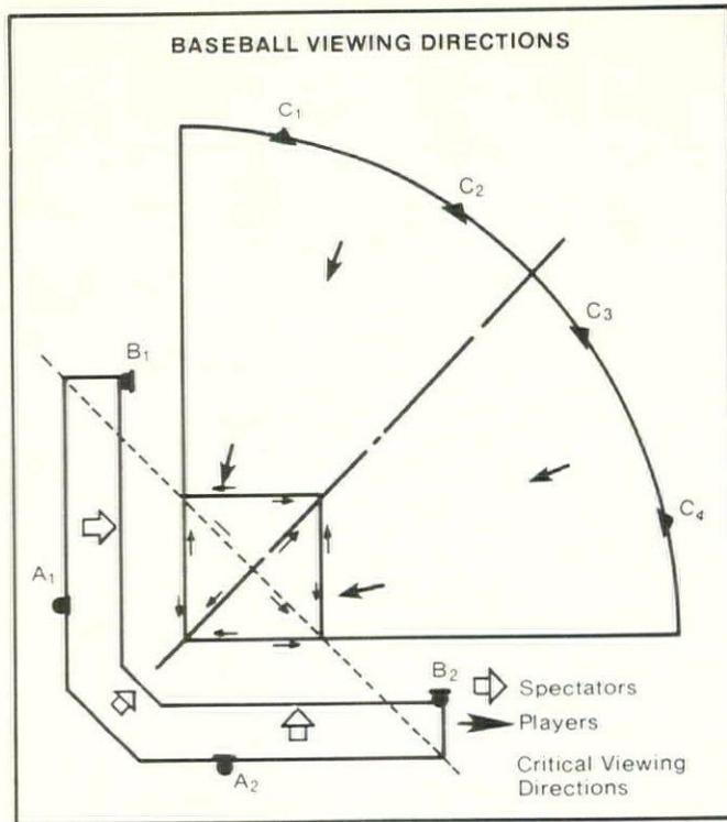
**FIELD OF BEAMS:** Poles should never be located directly in line with critical viewing directions. The A, B, C marks indicate pole locations.
