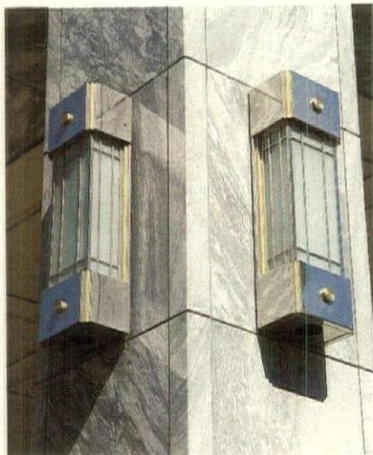
EXTERIOR WALL SCONCE, is 18 inches wide, 58 inches high, and has a 12-inch projection. The fixture is made of polished stainless and satin bronze. The frosted glass is backlit with two A lamps, and two 250-watt quartz lamps provide up and down light. Green Hiltcher, Shapiro of Chicago designed the fixture. Appleton Lamplighter, Appleton, WI. CIRCLE 62
