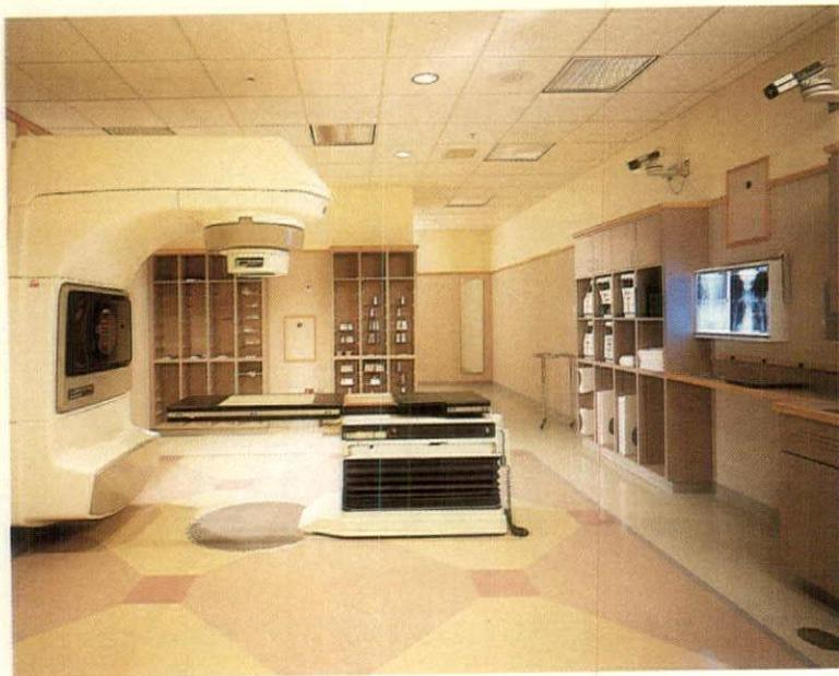
**THE HUMAN ELEMENT:** The radiation therapy room (above) was designed with the patient in mind—no lights are directly above the area of treatment. The lighting is a combination of fluorescent lamps (which operate at full intensity during pre-patient set up) and incandescent fixtures (which provide a warm touch).
