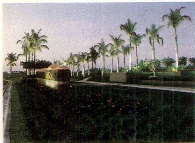
**THE RIGHT ANGLE:** Ground-mounted bullets housing R 38 metal halide lamps are aimed at 90-degree angles (right), along a 200-foot double row of palm trees (top), to maintain Sawgrass Park's upscale image in the evening (above).
