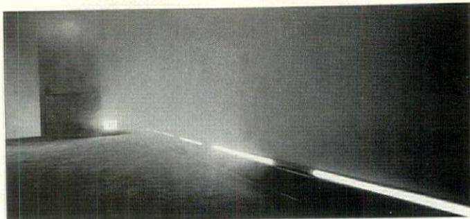
▶ **LOCTITE LIFELINE** emergency system provides low-level exit signs and path markings for higher visibility in smoke-filled areas. The system consists of emergency-activated electroluminescent light strips, which run along walls, and fiberglass-illuminated exit signs designed for placement 8 inches above the floor. Loctite Luminescent Systems Inc. **CIRCLE 57**
