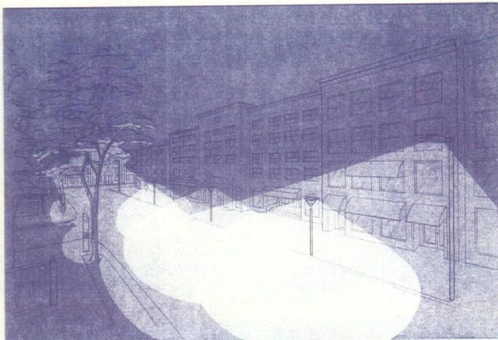
**TISSUE OVERLAY TECHNIQUE** provides a graphic, but not realistic view of a lighting scheme. In this drawing, the three layers of a street lighting approach are shown.
