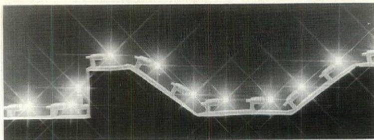
**LINEAR LIGHTING'S HORIZONTAL ACCENT LITE** uses a 5-watt, 12-volt quartz halogen lamp, and a 1-, 2-, or 4-watt, 24-volt incandescent lamp. It features a push button lamp ejector and compact design. The system can conform to indoor and outdoor configurations, and it is offered in spacings from 2 to 12 inches. Linear Lighting Corp., Long Island City, NY. **CIRCLE 70**
