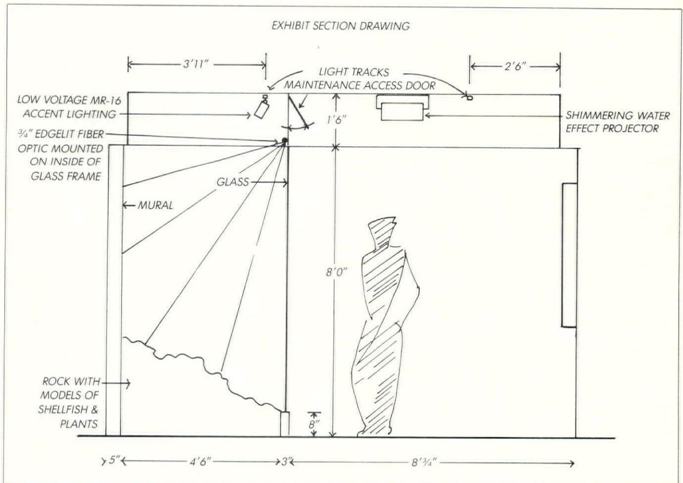
used for good color rendering, as well as excellent beam control. A combination of snoots, louvers, barndoors, linear spread lenses, and neutral density material focuses the light away from the background, and controls the intensity to create a progression from the bright, shallow end, to the shadowy, deep end.
