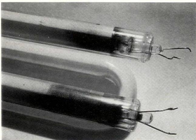
**FIGURE 1:** End of life occurs when insufficient material remains on the cathode. Cathode emissive material collects on the inner surface of the lamp, blackening the ends.
