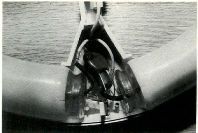
**FIGURE 6: A failed capacitor in a GE Circlite Miser lamp starter circuit.**
