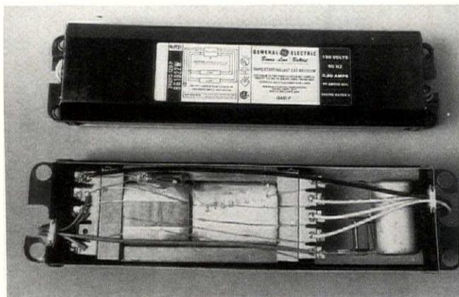
**FIGURE 3:** A core and coil electronic ballast photograph, courtesy of the General Electric Lamp Business Group.
