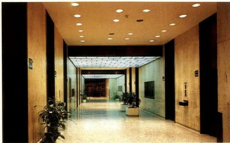
cavity are 60-watt A 19 silver bowl lamps. Recessed in the ceiling area between coffers are 150-watt PAR 38 floods.
