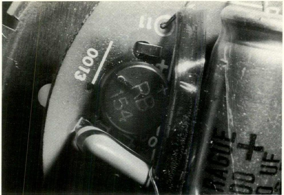
**FIGURE 4:** This input diode bridge opened, causing the failure in an electronic ballast.
