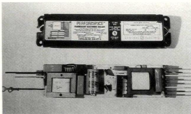
**FIGURE 2:** An electronic ballast photograph, courtesy of the General Electric Lamp Business Group.
