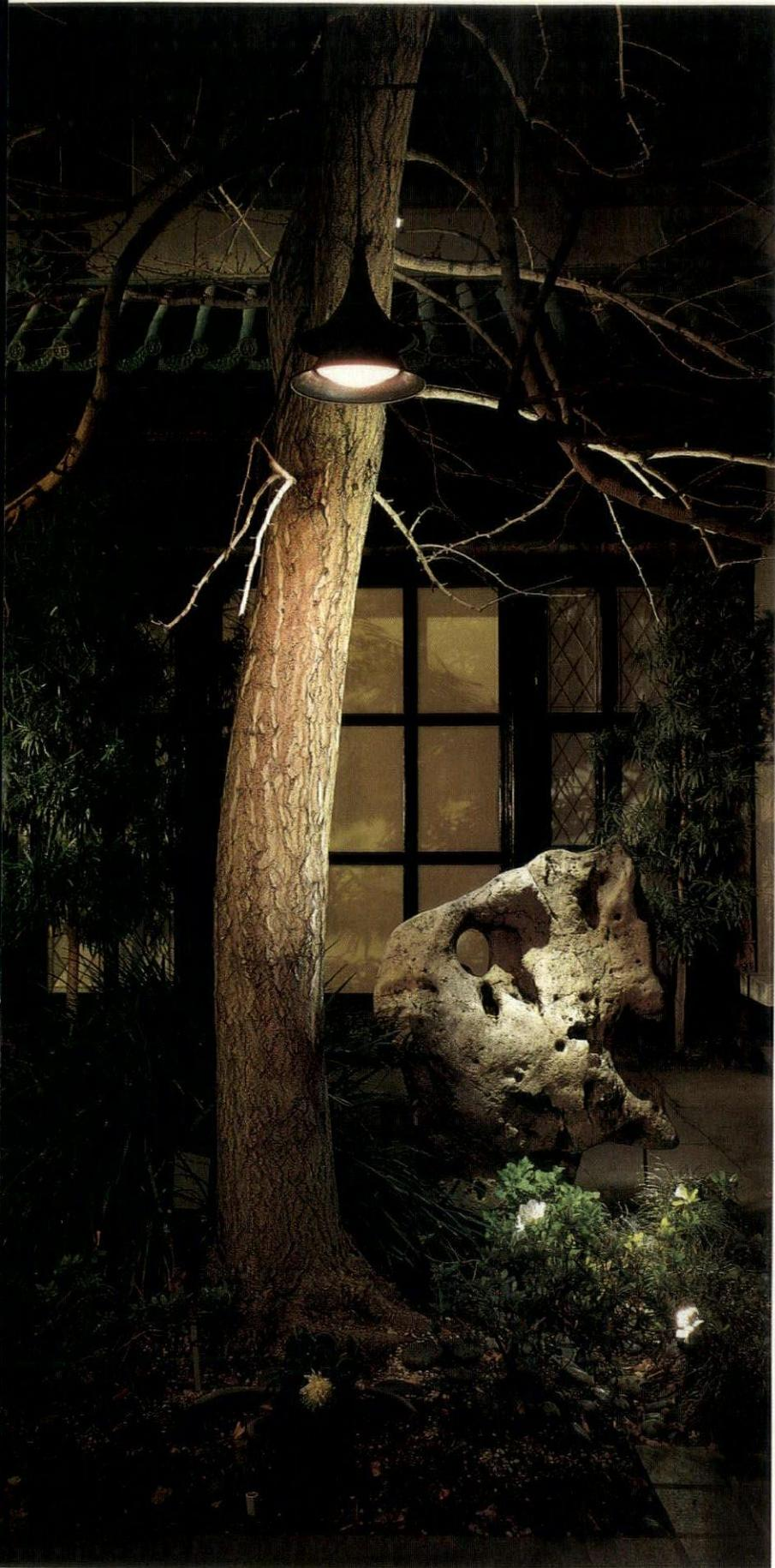
**RELAMPED LANTERNS:** Previously installed pendant fixtures that held 120-watt PAR lamps have been cleaned, rewired for low voltage, and relamped with 25-watt, 12-volt A-lamps.
