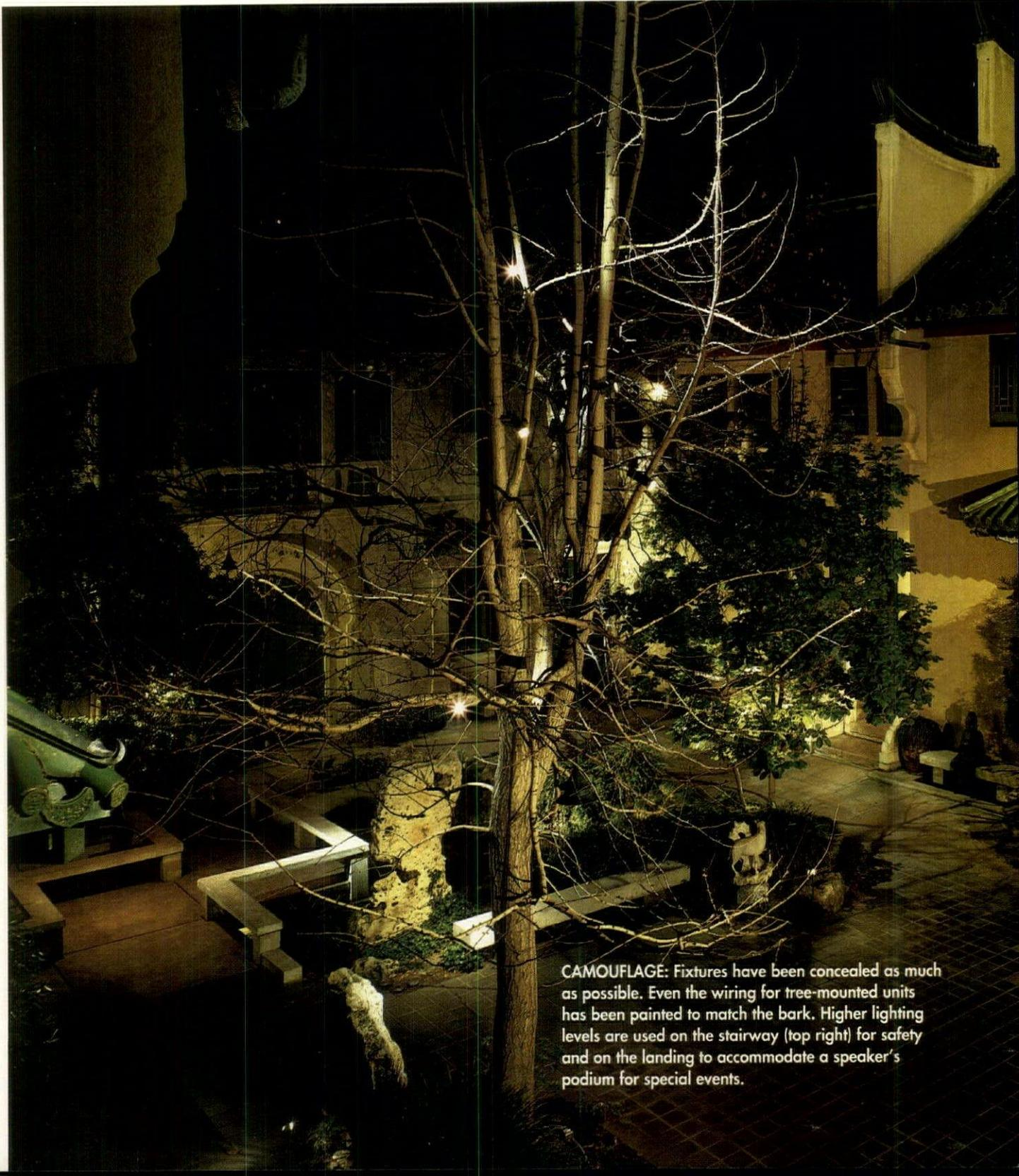
**CAMOUFLAGE:** Fixtures have been concealed as much as possible. Even the wiring for tree-mounted units has been painted to match the bark. Higher lighting levels are used on the stairway (top right) for safety and on the landing to accommodate a speaker's podium for special events.
