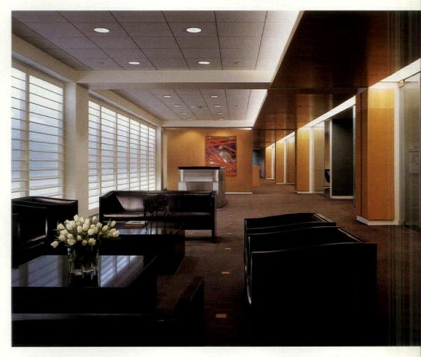
Light becomes a distinguished presence beginning in the reception area, where fluorescent lamps placed behind the brushed aluminum panels of the reception desk make them glow. Light is also emitted in the space between a horizontal yellow panel and the ceiling from which it is slightly dropped. "We were trying to make it appear as though there is a very intense source of light deep within the building that is looking for cracks from which to escape," says Kaplan.
