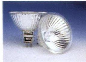
Capturing the infrared heat within the lamp capsule reduces the energy input required to bring the lamp up to optimal operating temperature, increasing operating efficiency. The new 37W Tru-Aim IR draws 13 fewer watts of power versus conventional 50W MR16 lamps.
