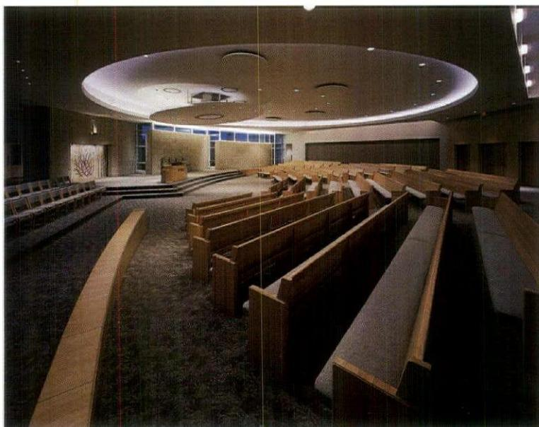
INSIDE THE SANCTUARY (LEFT), COLD CATHODE EMPHASIZES THE CIRCULAR CEILING COFFER AND THE SUSPENDED DISC. UNOBTUSIVE DOWNLIGHTS ILLUMINATE THE PEW AREA. SKYLIGHTS ENHANCED BY FLUORESCENT SCONCES LIGHT THE REAR.
