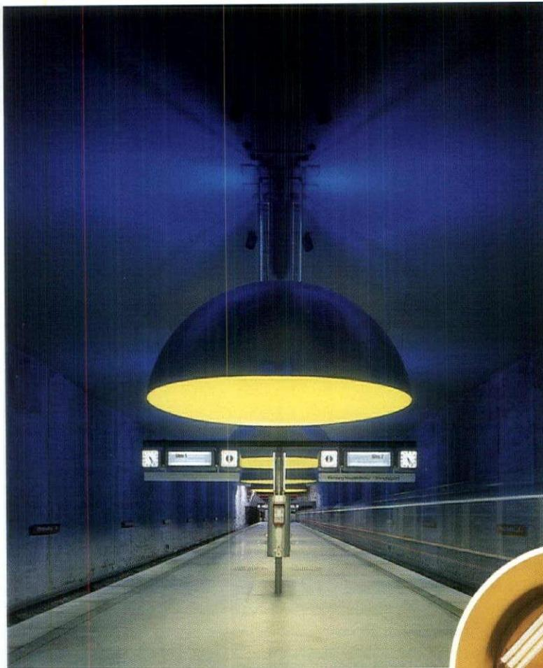
TWELVE 58W FLUORESCENT LAMPS WITH INTEGRAL REFLECTORS ARE MOUNTED IN A SQUARE FORMATION WITHIN THE HAND-FORGED ALUMINUM DOMES TO PRODUCE A 90-DEGREE BEAM OVER THE PLATFORM AND TRACKS.
