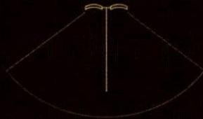
Sharp cutoff of lamp output eliminates trespass
