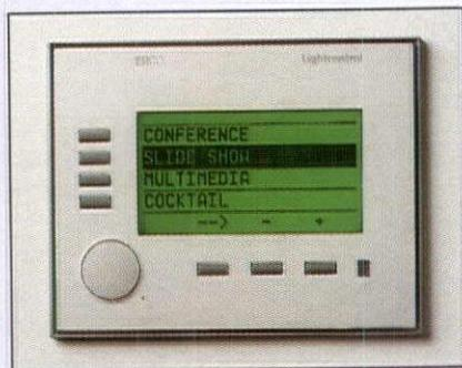
An infrared receiver is integrated into the preset. Extensions are connected directly to the bus control cable. When used with a PC interface and the V24 preset software, Lightcontrol can be operated from a PC. **Circle No. 95**
