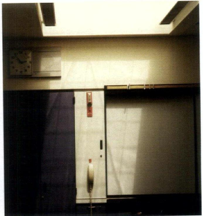
THIS CAPISTRANO CLASSROOM WITH A CLEAR SKYLIGHT ALLOWS DIRECT SUN AND UNCONTROLLED GLARE INTO THE SPACE AND CORRELATED WITH LOWER TEST SCORES.
