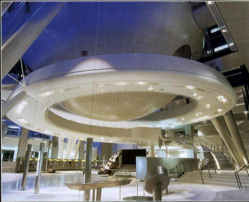
UNDERNEATH THE HAYDEN SPHERE (LEFT), THE HALL OF THE UNIVERSE IS ILLUMINATED BY TRACKLIGHTING MOUNTED ON THE UNDERSIDE OF THE COSMIC PATHWAY. A COMBINATION OF FLUORESCENT AND FIBER-OPTIC LIGHTING ILLUMINATES THE INTERACTIVE DISPLAYS.
