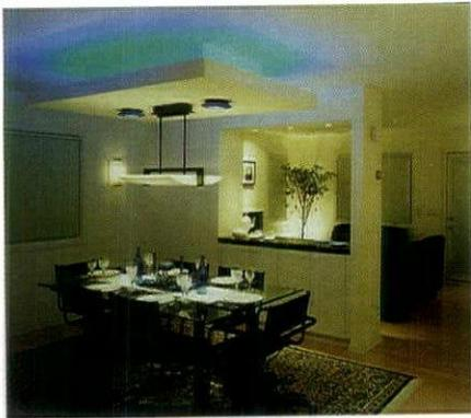
**FIGURE 6**—SIX DIFFERENT LAYERS COMBINE TO FORM A MULTI-USE LIGHTING SYSTEM IN THIS DINING AREA. CONTROLLED BY A PRESET SCENE CONTROLLER, THESE LAYERS CAN BE INDIVIDUALLY PROGRAMMED INTO MEMORY TO PROVIDE VARIOUS FUNCTIONS. PHOTO ©ROBERT J. EOVALDI
