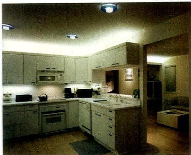
**FIGURE 1**—THIS KITCHEN USES A PREDOMINANTLY FLUORESCENT LIGHTING SYSTEM. UNDERCABINET T8 TASK LIGHTING IS COMBINED WITH SIDE-MOUNTED T8 STRIP FIXTURES FOR OVERCABINET INDIRECT LIGHTING ALONG WITH RECESSED BLUE GLASS LENS 13W COMPACT FLUORESCENT DOWNLIGHTS TO COMPRISE THE AMBIENT LAYER. PHOTO ©ROBERT J. EOVALDI
