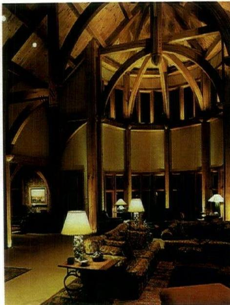
**FIGURE 7**—A COMBINATION OF TWO-TIERED UPLIGHTING FROM RECESSED FLOOR FIXTURES AT THE COLUMNS AND INDIRECT SCONCES AT THE UPPER WINDOW LEDGE COMBINES WITH DIRECT DOWNLIGHTING AND ART ACCENTING TO GIVE THE ARCHITECTURE THE EMPHASIS IT DESERVES. PHOTO ©ROBERT J. EOVALDI
