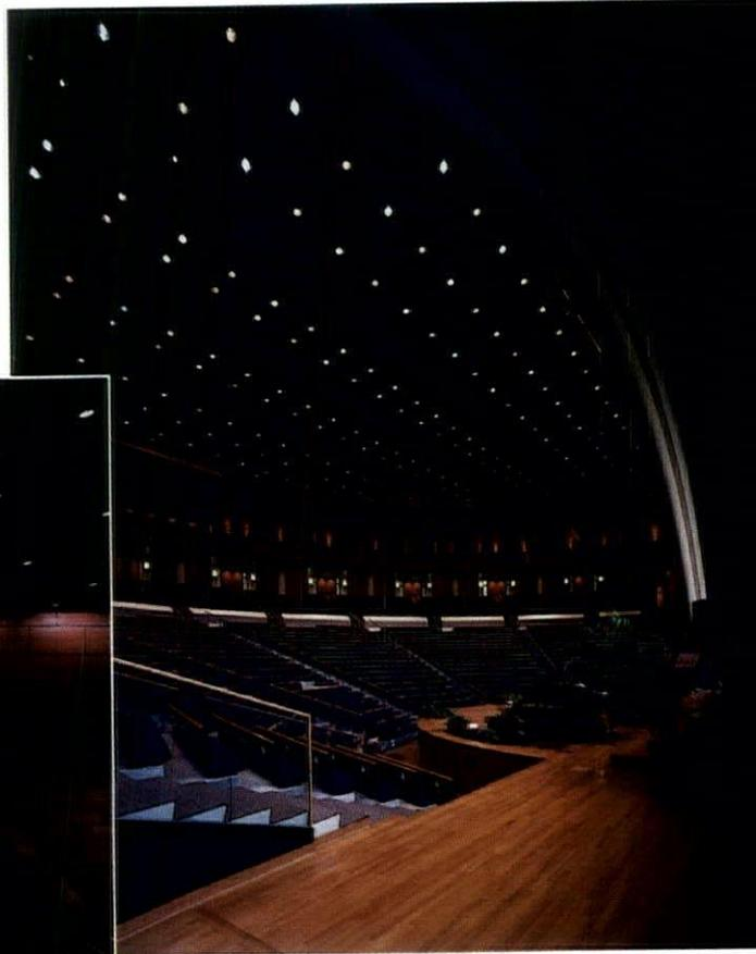
The 370 or so fixtures used throughout the space are connected to a dimming system, which can be adjusted to produce a maximum light level of about 68 fc during the day, balance with the level of daylight coming through the window. At night, the metal halides are turned off, with incandescents and fluorescents producing a light level about 21 fc. The connected load for the building is 6W/sq.
