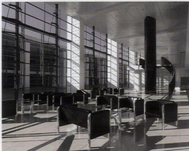
There is an ever-expanding box of tools where daylighting design is concerned. Radiance is a powerful software, capable of creating renderings like those above (Created by Graeme Watt of Synthesis Design & Visualisation Limited) that understand the interaction of sunlight with an architectural space. Other tools include heliodons (below) at places like the Southern California Lighting Technology Center.
