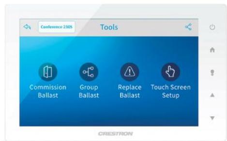
**GLDALI SpaceBuilder, Crestron** • This reconfigurable system is designed to control lighting in medium to large spaces. Its components are preprogrammed and shipped together. A startup module with a 7" touchscreen simplifies zone and sensor configurations. It controls up to 64 fixtures and up to 128 individual DALI ballasts or drivers. A maximum of four keypads, occupancy sensors, and open-loop daylight sensors can be added. • [crestron.com](http://crestron.com)
