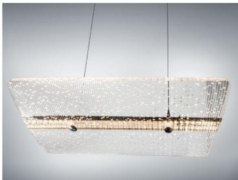
**Wing, Sensitile Systems** • This backlit suspended or wall-mounted luminaire delivers either direct or direct/indirect light and features LEDs that provide RGB and warm and cool white light. The fixture features an anodized aluminum housing and can be specified in 12" or 18" widths with single-fixture lengths ranging from 36" to 96". Power for the 12V fixture is provided either via direct wiring or wall outlet and it consumes 5W per foot. • [sensitile.com](http://sensitile.com)
