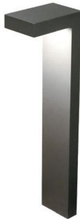
**Linea S, HessAmerica** • Emitting zero uplight at or above 90 degrees horizontal, this compact bollard is ideal for upscale residential and commercial areas, as well as applications concerned with light pollution. It comes in 24", 30", and 36" heights, with single or twin heads. Its LEDs deliver 3000K and 4000K with a CRI of 80-plus, while consuming 23W. The driver accepts 120V to 277V and offers optional dimming via zero-to-10V functionality. • [hessamerica.com](http://hessamerica.com)
