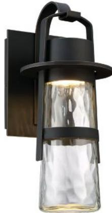
**Balthus LED Outdoor Luminaire, Modern Forms** • Available in 13<sup>1</sup>/<sub>4</sub>" and 16<sup>1</sup>/<sub>2</sub>" models, this LED sconce provides up to 481 lumens in 3000K with a CRI of 90. It has an oil-rubbed bronze finish and a mouth-blown, hammered clear glass diffuser. California Title 24-compliant and UL wet-location listed, the fixture dims with an electronic low-voltage dimmer. • [modernforms.com](http://modernforms.com)
