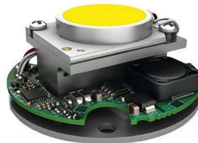
**XIM with Integrated Dimming Driver, Xicato** • This LED light engine integrates a dimming driver and uses onboard technology to monitor LED temperature and electronics, triggering a protection mode if the maximum temperature is exceeded. Available from 2700K to 4000K in a CRI of 83 or 98, it delivers from 1,300 lumens at 13.1W to 2,000 lumens at 21.2W. Dimming options include DALI and 1V-to-10V systems. A 48V, constant-voltage power supply is required. • [xicato.com](http://xicato.com)
