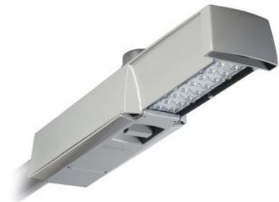
**MiniView Roadway, Philips** • This roadway lighting system delivers lumen packages of 2,700 to 5,500 to replace 70W to 100W high-intensity discharge fixtures. Designed to produce zero uplight, it is also fitted with side shields that limit light spill. The dimmable fixture's optics allow for wider pole spacing than is typical in the category, the company says. • [philips.com](http://philips.com)
