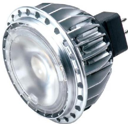
**MR16 Series TrueWhite LED Lamps, Cree** • Cree says its MR16 Series of LED lamps consumes up to 83% less energy than 50W halogens while offering a soft, glare-free diffused light. The lamp delivers more than 580 lumens in 3000K and has a CRI of 92. It is also available in 15-degree spot, 25-degree flood, and 40-degree wide flood beam angles, and is dimmable to 5%. A 1.97", ANSI-compliant form factor facilitates one-for-one lamp replacement. • [cree.com](http://cree.com)
