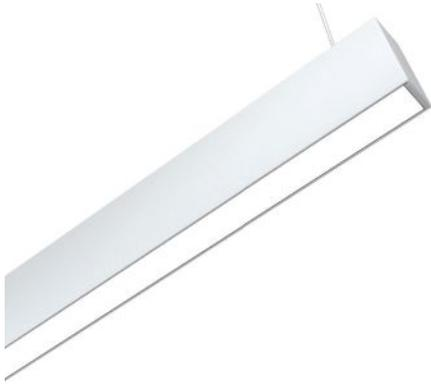
**Linea 1.5", Amerlux** • This linear LED luminaire with direct, indirect, and direct/indirect distributions is designed for use with a louver. Available in 2700K, 3000K, 3500K, or 4000K, the fixture comes in lengths of 47¾" and 95¾" with output options of either 5W or 10W per foot. Each luminaire can be suspended via aircraft cables or wall-mounted. An integral electronic constant current 120V-to-277V driver is standard with zero-to-10V dimming. • [amerlux.com](http://amerlux.com)
