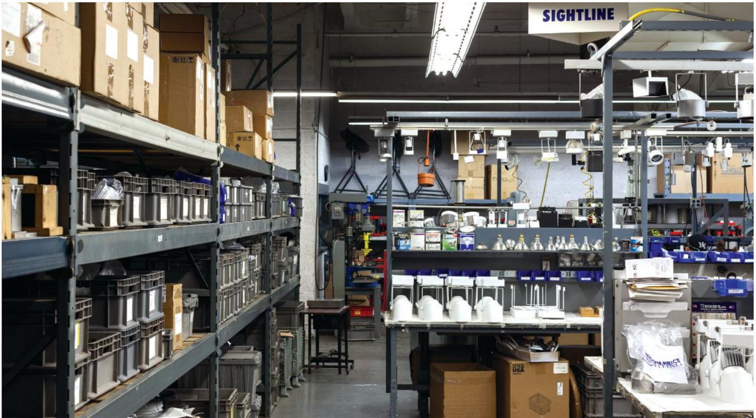
In the final assembly area at Edison Price's factory in Long Island City, N.Y., workers pair components that are made to order onsite with electronics that are sourced externally.
