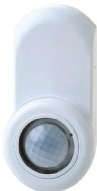
**Fixture Mount DALI Sensor, Enlighted** • This sensor turns conventional lamps into smart fixtures. Designed to fit in a 0.5" knockout in indoor fixtures, less than 0.28" of the sensor is visible once installed. The programmable device offers occupancy-, photo-, and thermal-sensing technology. With a 150' wireless range, it collects and communicates data to Enlighted's networked management systems. • [enlightedinc.com](http://enlightedinc.com)
