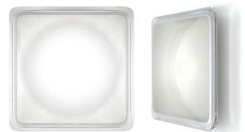
**Illusion, Luceplan** • Created by Argentine-born designer Francisco Gomez Paz, Illusion gives the impression of a sphere captured within a square—an optical effect created by the fixture's Fresnel lens and thermoplastic diffuser. The 9"-square fixture is suited for use indoors and can be mounted to the wall or ceiling. Dimmable, it is powered by a 3000K 17W LED module. • [luceplan.com](http://luceplan.com)
