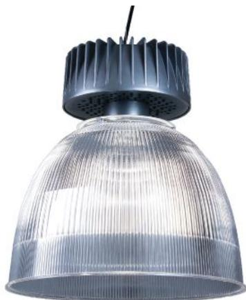
**Stellar Clear Prismatic LED Open Low-Bay, Delray Lighting** • This 16" diameter, dimmable low-bay downlight can mount to a standard J-box, suspend from an aircraft cable, or extend from a hard-stem pipe. It delivers up to 6,000 lumens and is available in 3000K, 3500K, or 4000K with a CRI of 92. The fixture is offered in 38W and 71W versions. Finish options are flat white, carbide black, and custom colors. • [delraylighting.com](http://delraylighting.com)
