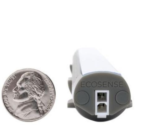
**Slim Cove INT, EcoSense Lighting** • This streamlined, line-voltage LED strip is suited for coves and other linear lighting applications and comes in 6", 12", and 48" lengths. Available in 2700K, 3000K, 3500K, or 4000K with a CRI of 80-plus, the luminaire consumes 3.5W per foot and has a 120-degree square beam spread. It measures 1.37" wide and 0.93" tall with mounting clips and a polycarbonate housing and lens. • [ecosenselighting.com](http://ecosenselighting.com)
