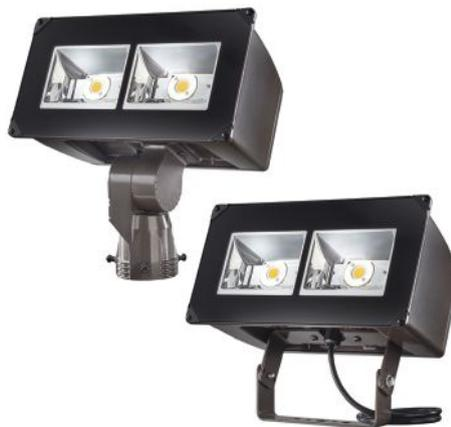
**Night Falcon, Eaton's Cooper Lighting/Lumark** • Available in packages of 9,400 and 14,600 lumens, this floodlight is suited for illuminating building façades, signs, and exterior vertical displays. It is offered in 4000K, as well as 3000K and 5700K, all with a minimum CRI of 70. UL wet-location listed and IP66-rated, the fixture has a weather-resistant finish and comes with two mounting options. • [cooperindustries.com](http://cooperindustries.com)
