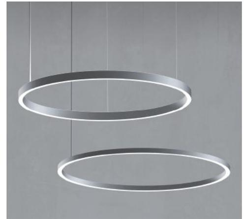
**Uno and Duo LED Pendants, Delray Lighting** • These circular LED suspension fixtures are available in direct (Uno) or direct/indirect (Duo) light distributions. Composed of slender extruded aluminum hoops—Uno measures 1" wide by 1" tall while Duo measures 1" wide by 2" tall—in 2', 4', and 5' diameters, the fixture is intended for low-ceiling spaces. Available in 3000K and 3500K with a CRI of 90. • [delraylighting.com](http://delraylighting.com)
