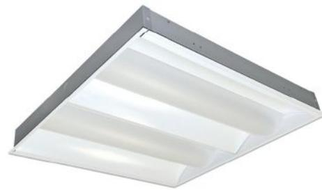
**R1L/R2L Series, LaMar Lighting** • Measuring less than 3" deep, this series of recessed ceiling troffers comes in 2x2, 1x4, and 2x4 sizes and is suited for use in a standard 15¼" inverted T-bar grid and shallow plenum locations. Offered in 4000K, the fixture can also be specified in 3500K and 5000K. The series provides 2,000 lumens from the 2x2 size with a CRI of 80-plus. All fixtures are designed to replace a 32W to 34W fluorescent. • [lamarlighting.com](http://lamarlighting.com)
