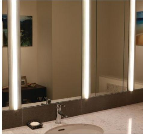
**Reflections V, Dreamscape Lighting** • This semi-recessed, linear LED wall luminaire is designed to illuminate bathroom vanities. Available in 3000K with a CRI of 97, the fixture is housed in an extruded aluminum frame with a curved lens that can be used alone or placed between sections of a 1/4"-thick mirror. Fixture lengths can be specified to meet dimensional requirements. • [dreamscapelighting.com](http://dreamscapelighting.com)
