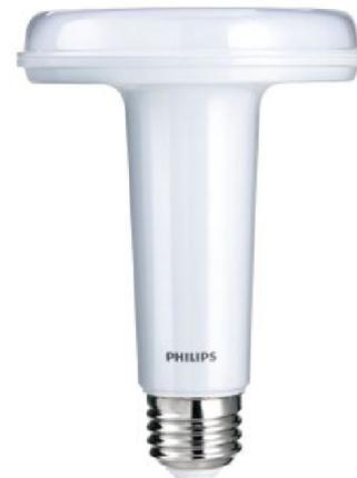
**SlimStyle BR30, Philips** • This indoor BR30 LED lamp replaces 65W incandescent floodlights. Its thin form factor offers uniform light distribution while conducting heat away from the LEDs to require a minimal heat sink. Consuming 9.5W to produce 650 lumens in 5000K, the dimmable lamp fits an E26 base and uses 85% less energy than its incandescent predecessor, according to Philips. • [philips.com](http://philips.com)
