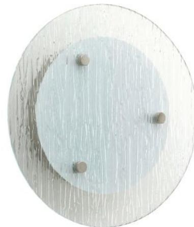
**Beyond, Hubbell Lighting/Progress Lighting** • The Beyond series from Progress Lighting comes in round (shown) and square profiles with options for textured glass, metallic overlays, and geometric acrylic diffusers. Mounted to the walls or ceiling, the 120V fixture measures 12" in diameter and 6" deep, and is offered with a replaceable 17W LED module in 3000K with a CRI of 90. • [progresslighting.com](http://progresslighting.com)
