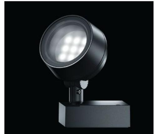
**Gecko, Erco** • Measuring 9<sup>7</sup>/<sub>8</sub>" from base to top, this compact luminaire offers six light distributions for use illuminating façades, entryways, monuments, and within parks. High-powered 8W to 18W LEDs provide 3000K or 4000K. A slightly conical head rotates 360 degrees and tilts 130 degrees for precise positioning. The fixture is IP65-rated and features a non-reflective safety glass lens. • [erco.com](http://erco.com)
