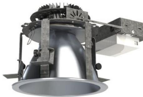
**LRD3, LumenOptix** • LumenOptix is growing its family of retrofit downlights with this series of 15W to 95W commercial LED fixtures designed to replace 250W and 500W quartz-halogen and 250W and 400W metal halide downlights. Lumen packages from 1,000 to 8,000 lumens are available. Designed for use in spaces with ceiling heights up to 50', the open-architecture platform comes with more than 40 LED module options, optics, finishes, and aperture sizes. • [lumenoptix.com](http://lumenoptix.com)
