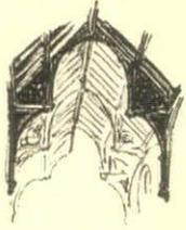
Hammer Beam Truss is not a truss but an arch
