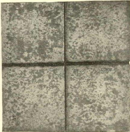
This section of concrete flooring was stained with Oak Leaf Brown. Note the color gradations and Duotone effects due to variation in the cement's lime content and density of surface.
