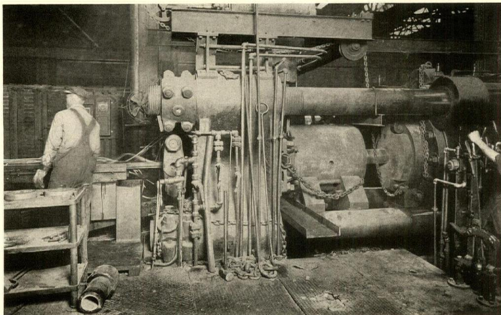
*One of man's newer machines, which extrudes molten metal through a die in such profiles as may be desired. At present we use this machine to imitate forms originating in wood or stone construction*
