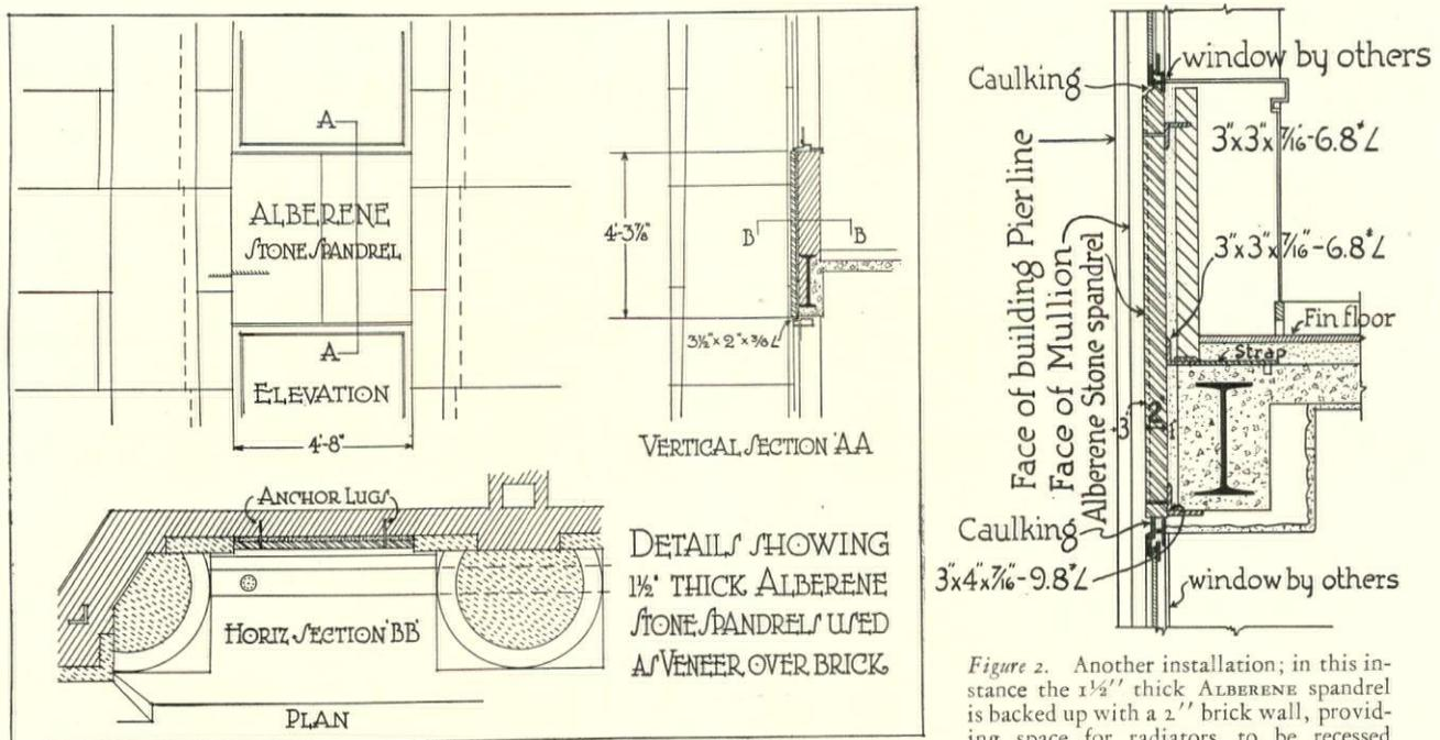
Figure 1. ALBERENE STONE SPANDRELS as installed on the 32nd and 33rd floors of the Newark & Essex Bank Building
