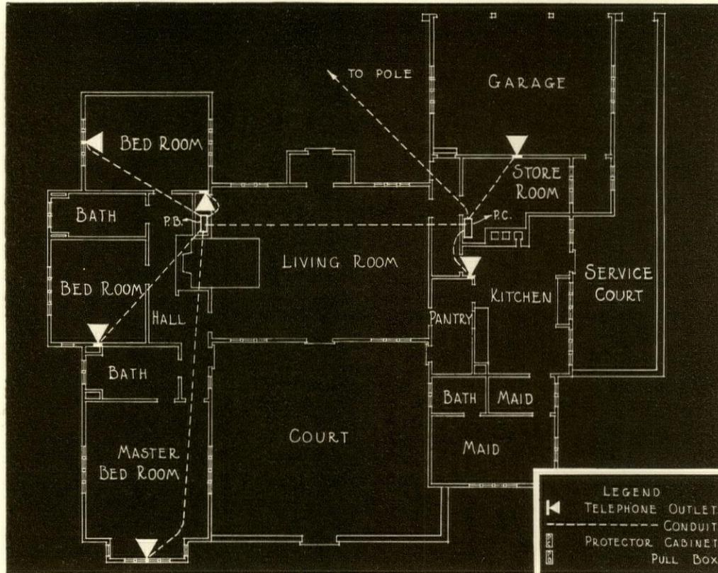
Complete telephone convenience is provided in the residence of Dr. George W. Hawley, Bridgeport, Connecticut, by six telephone outlets, including one in the garage. The telephone wiring is carried in conduit hidden in the walls and floors. FRED C. JOHNSON, Architect, Bridgeport.
