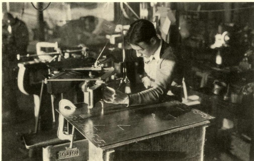
*Another of man's newer machines which transfers, by means of a pantograph, a design on a master plate to a blank sheet, routing it to the desired depth*
