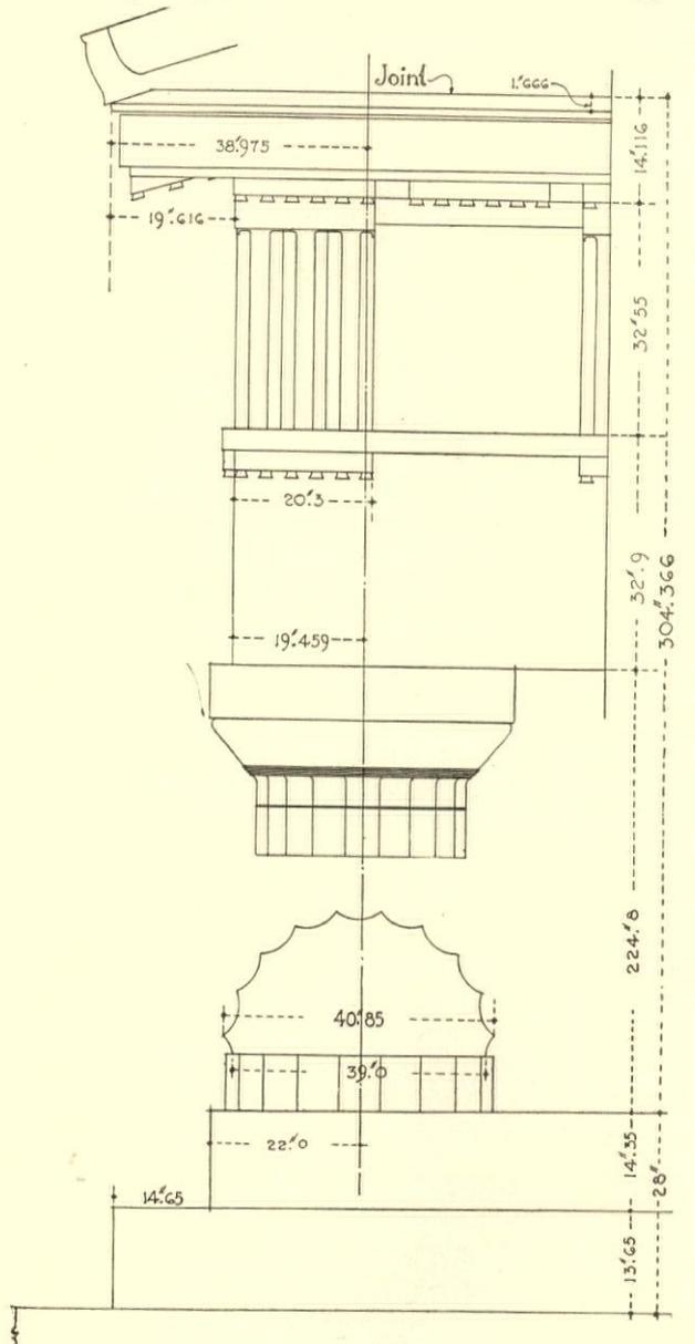
FIG. 3. Temple of Theseus: Detail of the Order, from Stuart and Revett, with figures in inches
