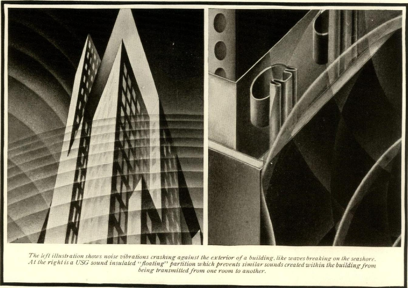
The left illustration shows noise vibrations crashing against the exterior of a building, like waves breaking on the seashore. At the right is a USG sound insulated "floating" partition which prevents similar sounds created within the building from being transmitted from one room to another.
