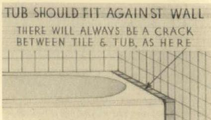
ing a band of split tile to be run between the tub and the wall. The architect should ask for, and get, the roughing size of the tub. This will enable him to do his part in laying out a workmanlike job of the bathroom.
