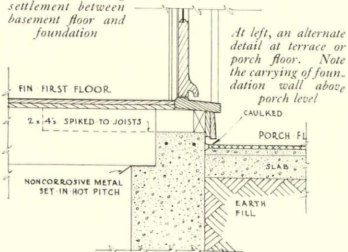
At left, an alternate detail at terrace or porch floor. Note the carrying of foundation wall above porch level
