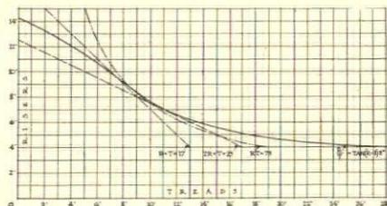
Fig. 2 (repeating Fig. 1 of Part I). The curve of Fig. 1 plotted to show its relation to the straight-line representations of the three old rules
