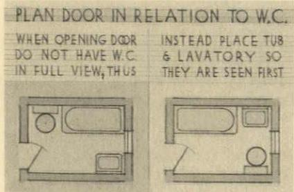
other item in the layout is the swing and position of the door. It is desirable to have it so placed that upon opening it, the water-closet is not in full view.
