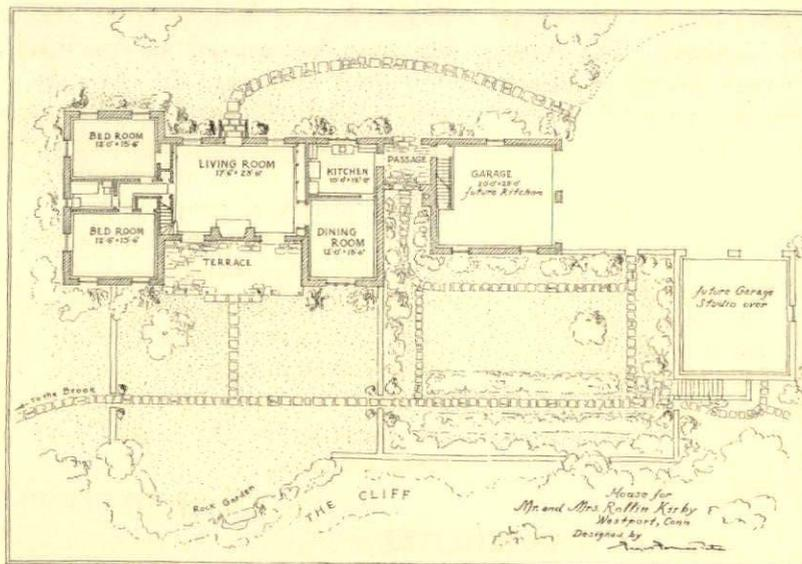
The house is built of native field stone, whitewashed. It has steel casement windows, painted black, a black slate roof, and black trim. The window boxes are sea green. The plan shows the house as originally built. The present dining-room is to be enlarged to take in
