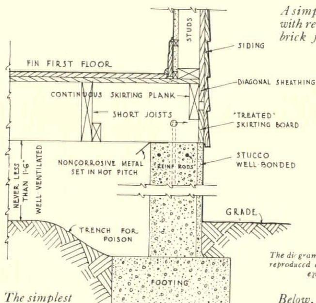
*A simple method of capping foundation wall with reinforced concrete strip where stone or brick facing is used—otherwise metal cap should extend through wall*
