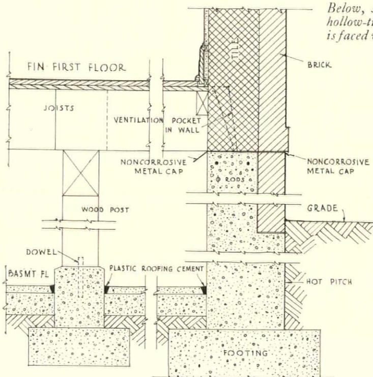
Below, standard masonry construction with hollow-tile exterior wall. If foundation wall is faced with brick or stone, metal strip should extend through wall
