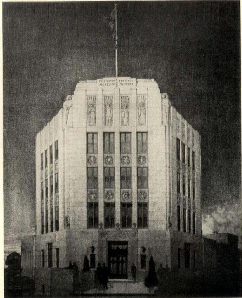
*The architect's preliminary perspective study of the building as seen from the south. In the cast stone resembling granite a pinkish tint relieves it, and the base is darker than the walls above*
