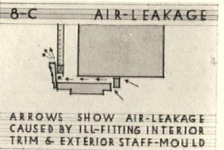
ARROWS SHOW AIR-LEAKAGE CAUSED BY ILL-FITTING INTERIOR TRIM & EXTERIOR STAFF-MOULD
