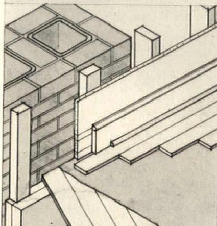
WITH FURRING — PLASTER IS LESS LIKELY TO CRACK FROM MOVEMENT
