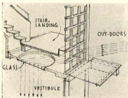
through prism-glass windows under a stair landing. Electric lights in this space light the vestibule at night.
