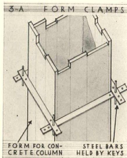
adequate support without stretching (Fig. 3A).
