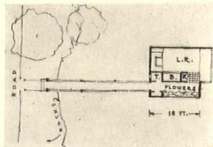
lished by a small suspension bridge, but the local building department insisted upon a straight span of wooden construction. The superstructure on the column is also entirely of wood, stained dark. Folding glass doors separate the living-room from the additional overhang of the balcony. "B" on the plan represents a pair of bunks, upper and lower. It seems to us that the architect should have provided a drawbridge.
