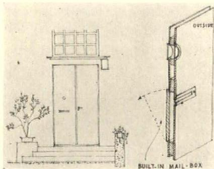
tred above its slot is a peep hole. The construction of both of these accessories is shown in the section.
