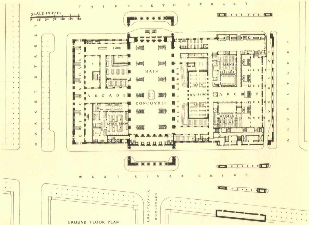
*Above, ground-floor plan of the terminal. Below, plan showing the relationship among the Terminal west of the Schuylkill River, the centre of Philadelphia, the Parkway, and the Pennsylvania Boulevard still to be built*
