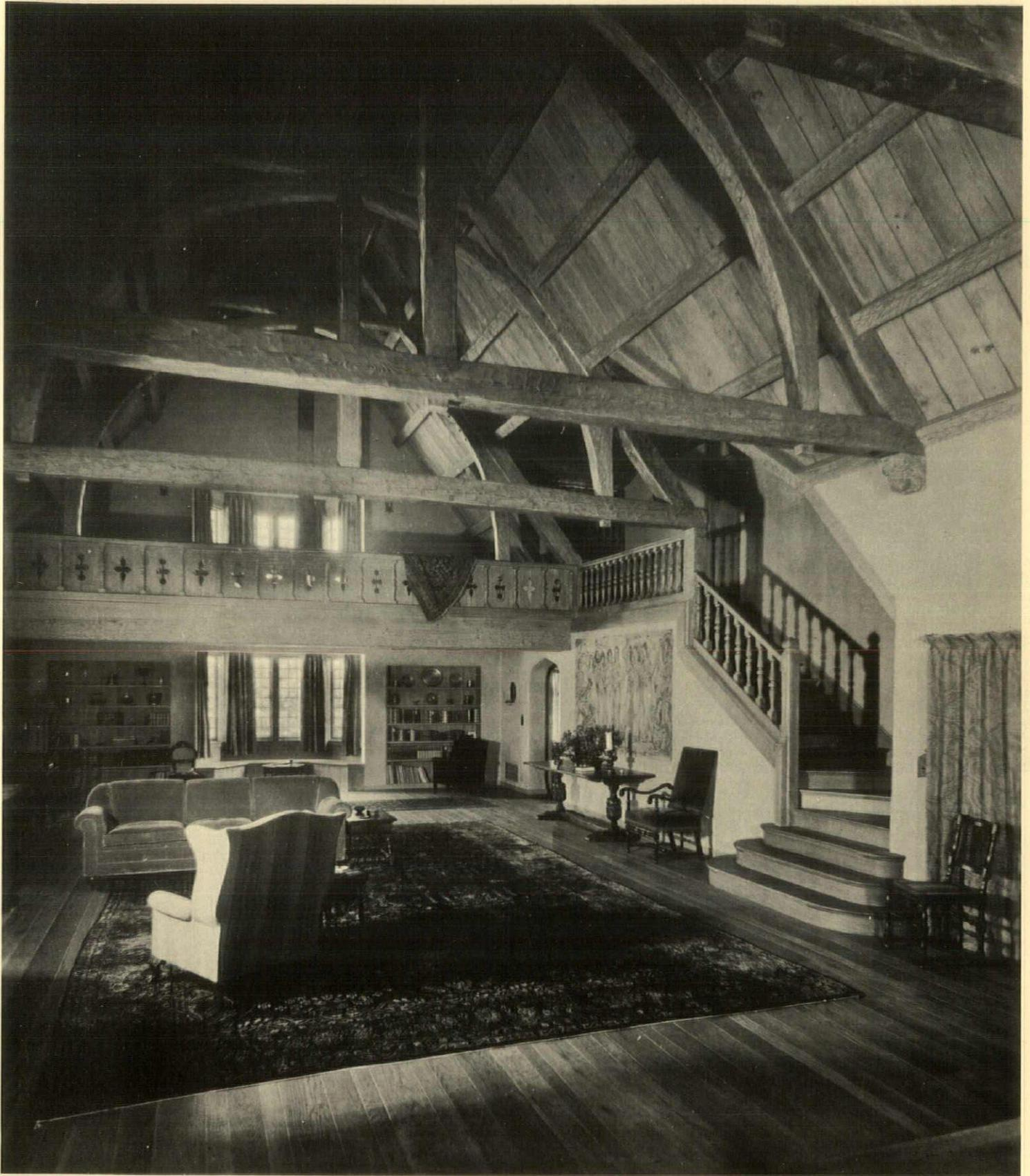
*The oak timbering of the studio has been given a color about like that of driftwood. Floors are of heavy oak plank in random widths*
