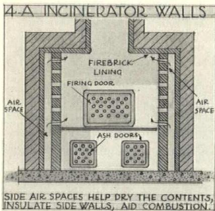
In laying out the incinerator, it is well for the architect to consult the manufacturer of several types, so that he may be well advised on the more essential points of the construction. The destructor should be large enough to take the accumulation of rubbish during at least one day, preferably two.
