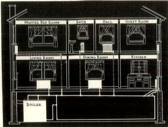
This shows you how simple the Burnham Unit-Air Conditioner System is. The Unit-Air Conditioners are located in the living and dining rooms downstairs and the master bedroom upstairs. Rest of heating done by the Burnham Slenderized Radiators.
