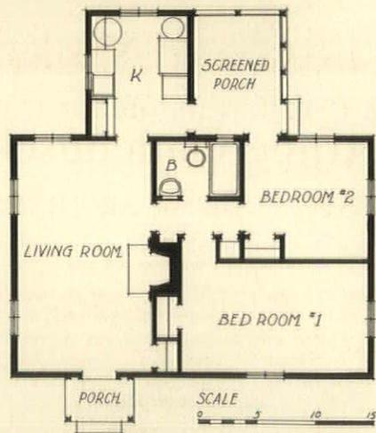
*Wood frame on brick foundation. Interiors, plaster on metal lath. Exterior walls and exposed ceilings are insulated with glass wool. The house is fully electrified, including the heating. Cost, not including overhead, \$4359*
