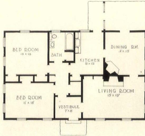
pine boards are used for flooring, treated with a dark stain filler and covered with dull-surface varnish. As to size, the house contains 17,835 cu. ft., and the cost was \$4000
