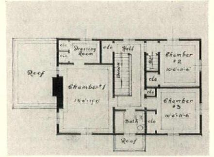
*is faced with shiplap, the house is shingled and painted white, with dark green shutters and roof. Cubage, approximately 30,000 cu. ft.; cost, about 34 cents per cu. ft. Away from the New York area the architect has built similar work for 32 cents per cu. ft.*
