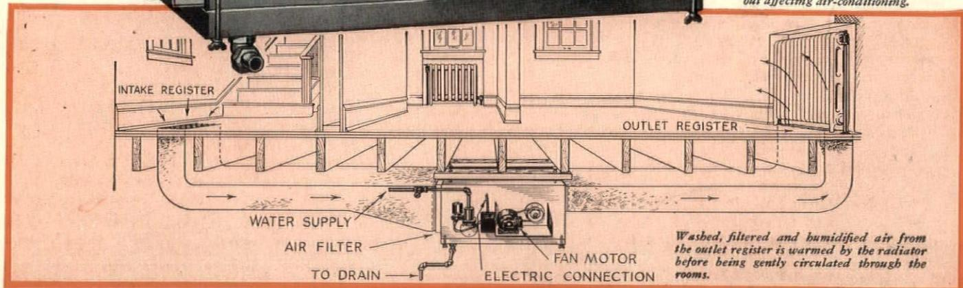
Washed, filtered and humidified air from the outlet register is warmed by the radiator before being gently circulated through the rooms.
