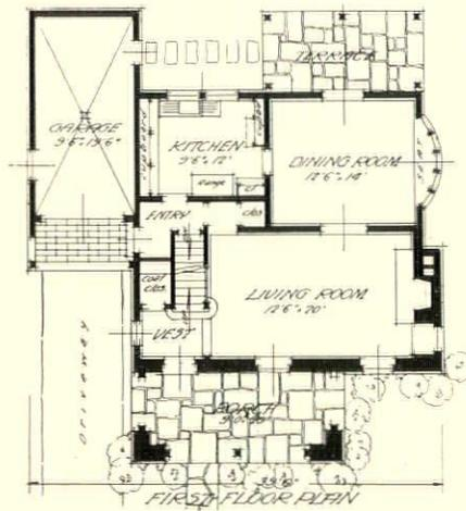
The house contains 27,900 cu. ft., and cost \$8900, or about 32 cents per cu. ft. There is a full cellar under it. Front wall and porch are of Pennsylvania ledge stone, the other walls of frame construction covered by stucco and shingles. The roof is of slate, and is insulated. Inside, the baths are tiled, other floors oak, with the exception of linoleum in the kitchen
