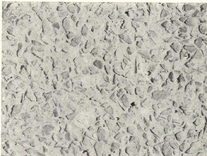
FIG. 4.—SURFACE OF WASHED CONCRETE.
