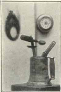
In this test the flame of a powerful blow-torch was placed within two inches of J-M Asbestos Roofing. At the end of fifty minutes the roofing was not burned or injured, being only slightly blackened with smoke.
