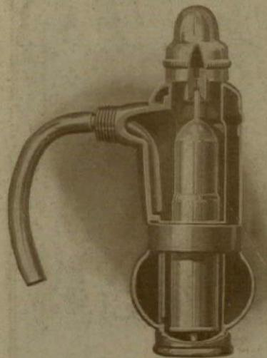
Inner view of Norwall Siphon Air Valve, showing simple and compact construction. The sole motive force is the expansion and contraction of the air in the outer chamber acting on the surface of the water of condensation in the valve. When flooded the Siphon returns the surplus water to the radiator.
