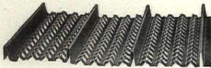
Thin concrete roofs, light in weight, are made by merely laying the HY-RIB over the supports and pouring on the concrete.
