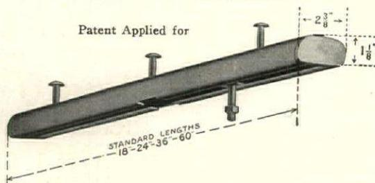
Manufactured from the highest grade of pressed steel and suitable for  $\frac{5}{8}$ " or  $\frac{3}{4}$ " bolts. Only  $1\frac{1}{8}$ " deep, permitting reinforcing steel to pass over it without reducing the strength of the construction.
