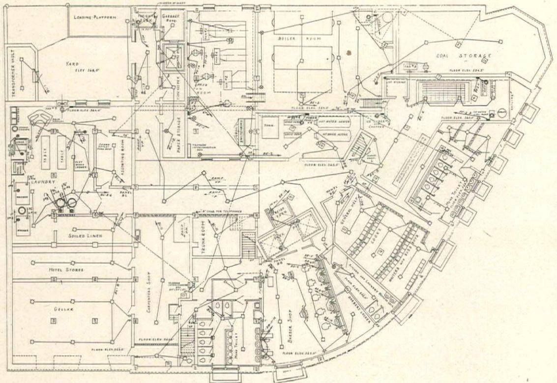
Electric Wiring Plan, Basement, The Niagara, Niagara Falls, N. Y.
