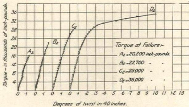
Fig. 5. Torque-Twist Curves for 5 x 7 1/2 in. Specimens
