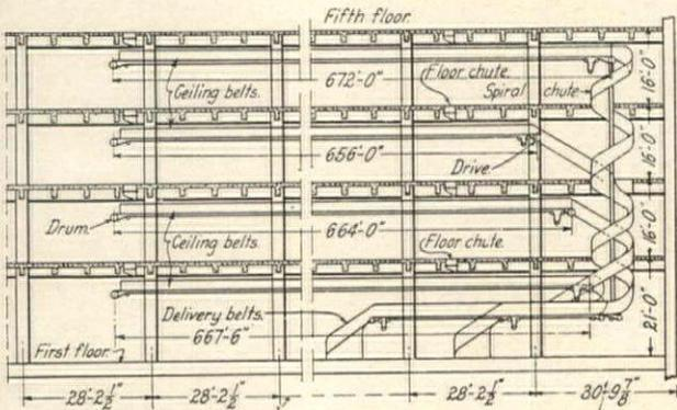
A part longitudinal section, showing how the ceiling belts deliver mail to the spiral chutes
