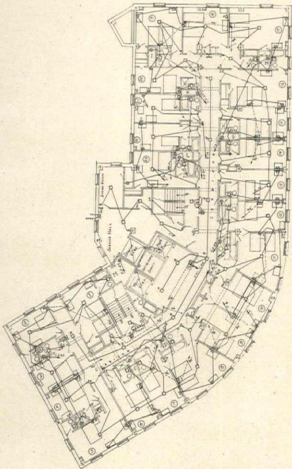
Electric Wiring Plan, Typical Floor,
