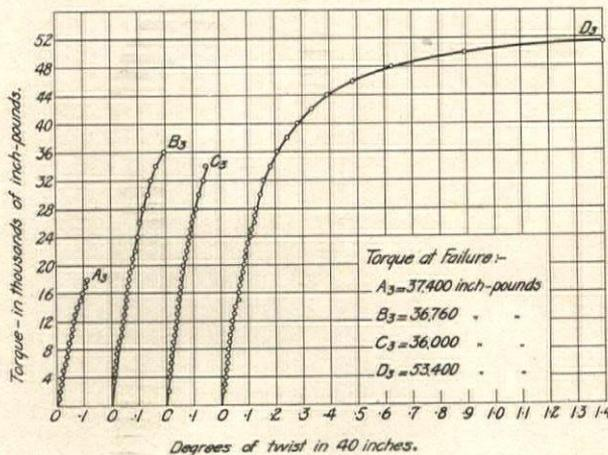
Fig. 6. Torque-Twist Curves for 5 x 10 in. Specimens
