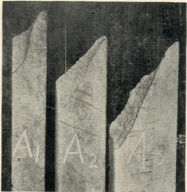
Fig. 2. Torsional Fracture of Rectangular Specimens of Plain Concrete
