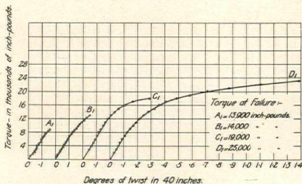
Fig. 4. Torque-Twist Curves for 5 x 5 in. Specimens, Plain and Various Reinforced
