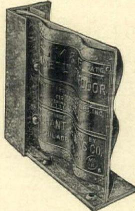
A double panel of heavy corrugated galvanized steel, lined with sheet asbestos and bound in a rigid continuous frame of bar steel, the M & E "Almetl" Fire Door protects better, stands harder knocks, lasts longer and pays for itself in insurance reductions—yet costs no more than the ordinary kind.
