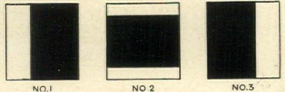
The three squares shown above indicate the relative performance of Rib Strip and Monarch No. 400 Strip on thirty double-hung windows having a total crack perimeter (the opening between the sash and the frame through which cold air infiltrates) of 630 lineal feet—outside wind velocity 15 miles per hour.
