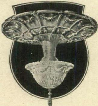
**MAZE-LITE**—Reflector 12½ inches diameter. Bowl 6¼ inches diameter, designed for 100, 150 watt lamps. Maze-Lite distributes its light evenly to the ceiling and coves of the room without bright spots on the ceiling. A pleasing, restful touch of color is provided in its ivory tinted bowl.
