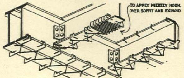
An important point about Standardized Metal Caging is that it always extends into the lower corners of the soffit, giving firm support at the point where heat usually causes the first disintegration of the concrete. A beam encased in concrete, held in place by S. M. C., is perfectly and permanently fire-proofed — its concrete covering has maximum fire-resistance.
