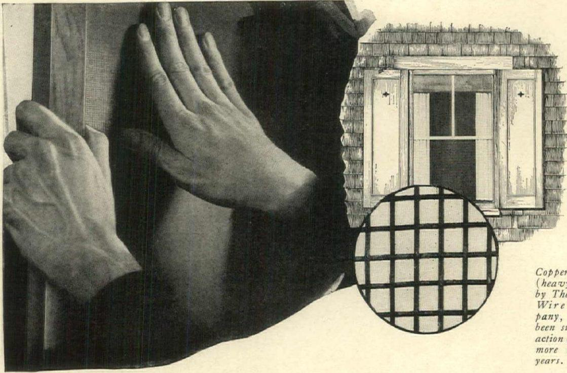
*Copper Screen Cloth (heavy grade) made by The New Jersey Wire Cloth Company, which has been subjected to the action of salt air for more than twelve years.*
