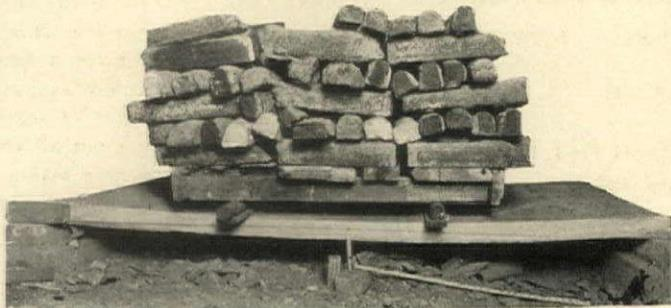
This Gunitite slab has a span of 8', a width of 4', and a thickness of 3 1/4". It is reinforced with expanded metal. The load mentioned was placed on it 29 days after it was shot and the deflection at that time was 29/32". On July 17th, 1920, 70 days later, the deflection was 1 3/4". On May 5th, 1922 the deflection was 2" and there has been no increase in deflection or cracking since.
